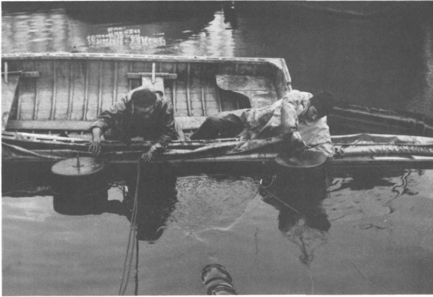
PLATE 11 (a) LEVEL ADJUSTMENTS OF THE SKIMMER DURING TESTS
