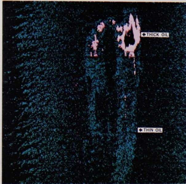
MSS Thematic Colour Image MSS 3, MSS 6, MSS 8, MSS IR Wallops Oil Spill C - GRSA Flight Line 2 November 3, 1978 16:27:51 GMT
