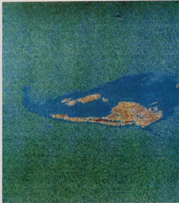
FIGURE 76 DCLS, WALLOPS OIL SPILL. Superposition of UV and IR colour enhanced images. C-GRSC Flight Line 6, November 2, 1978.
