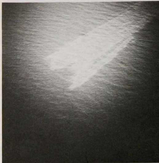
Vinten 70mm Camera with UV Filter 2405 Double-X Aerographic Film Wallops Oil Spill C-GRSA Flight Line 22 November 3, 1978 17:50:17 GMT
