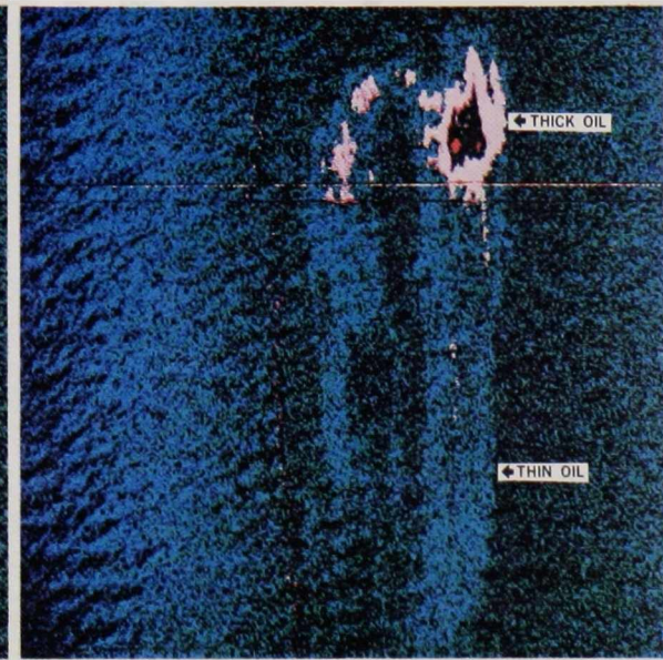
MSS Thematic Colour Image MSS 3, MSS IR Wallops Oil Spill C - GRSA Flight Line 2 November 3, 1978 16:27:51 GMT
