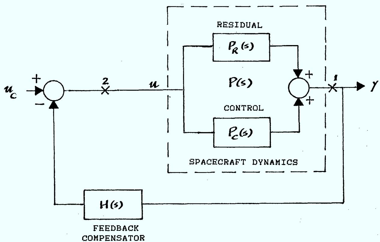
FIGURE 5-2 A Control System Representation for Flexible Spacecraft
