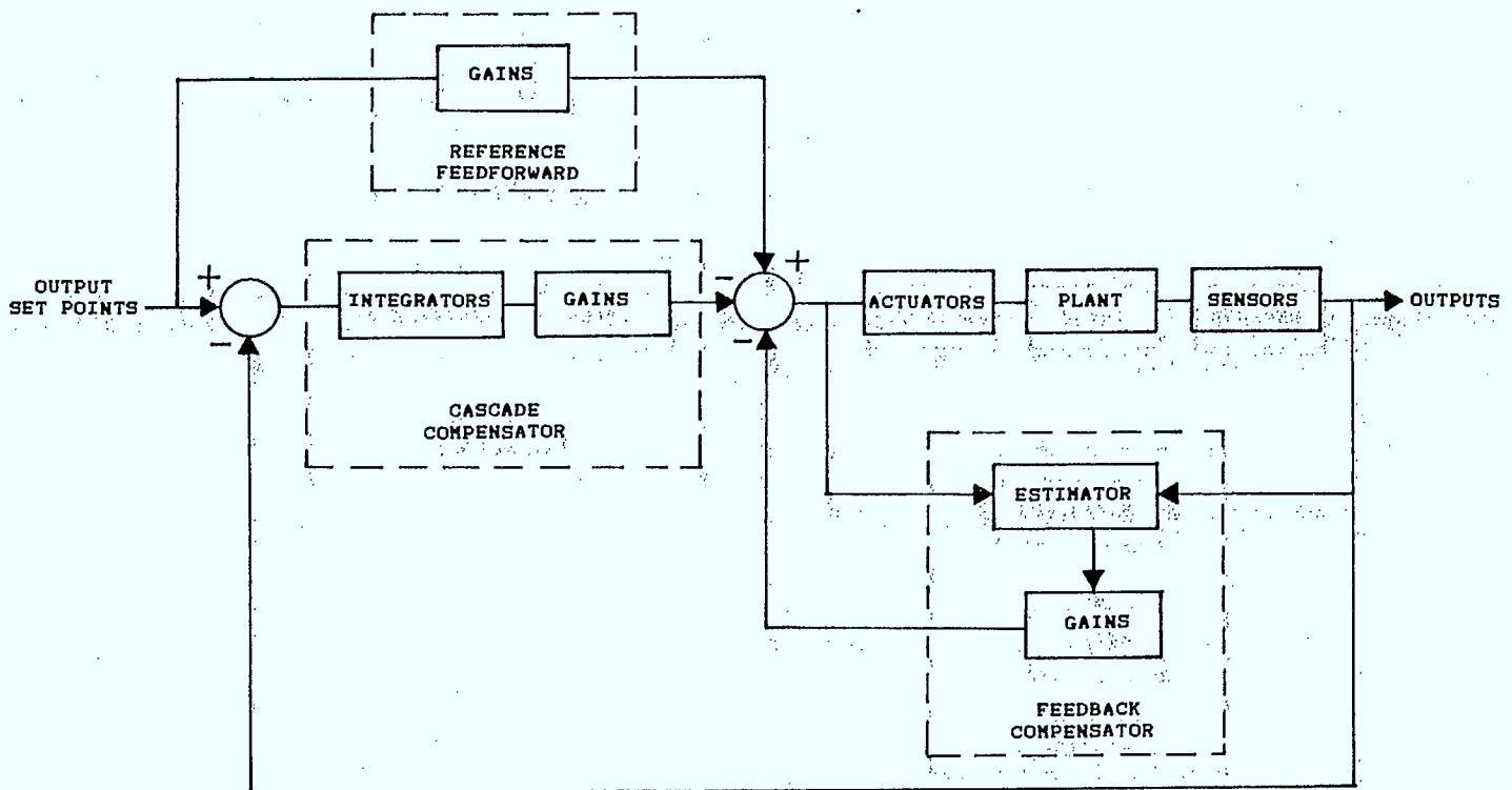
FIGURE 4-1 Partitioned Configuration of Tracking Compensator
