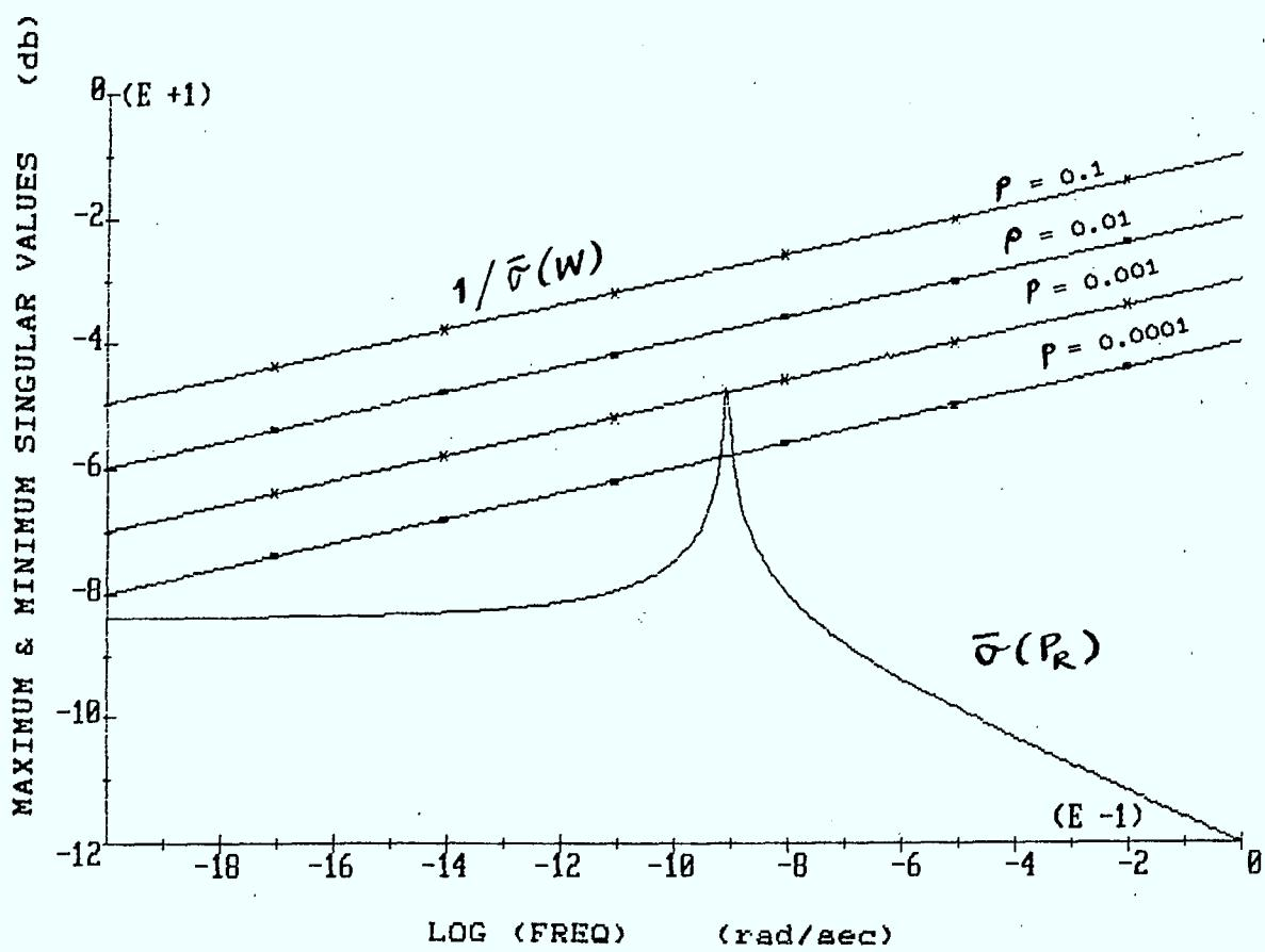
FIGURE 5-4 Design Iteration Using Robustness Criterion (5-16)
