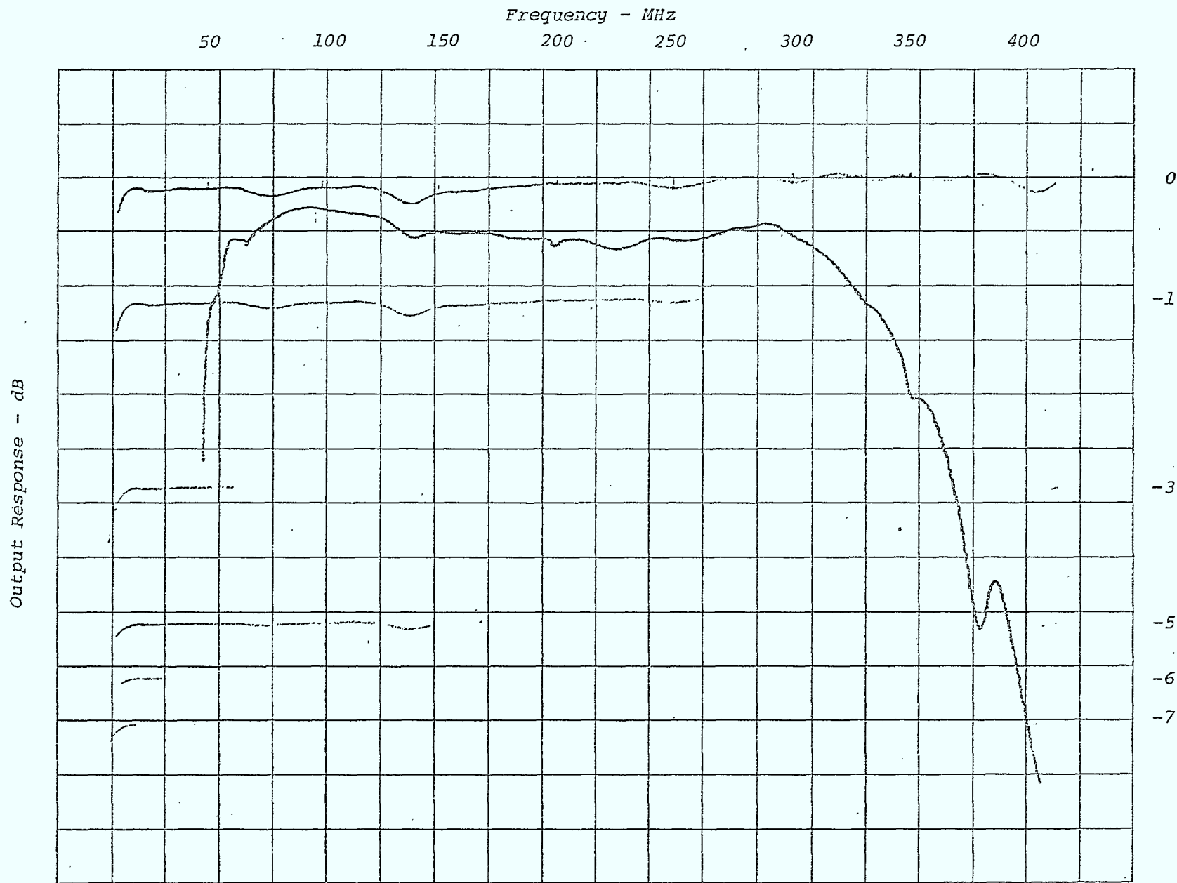
Figure 8 -Frequency Response of Starline 300 Trunk Amplifiers with Diplex Filters
