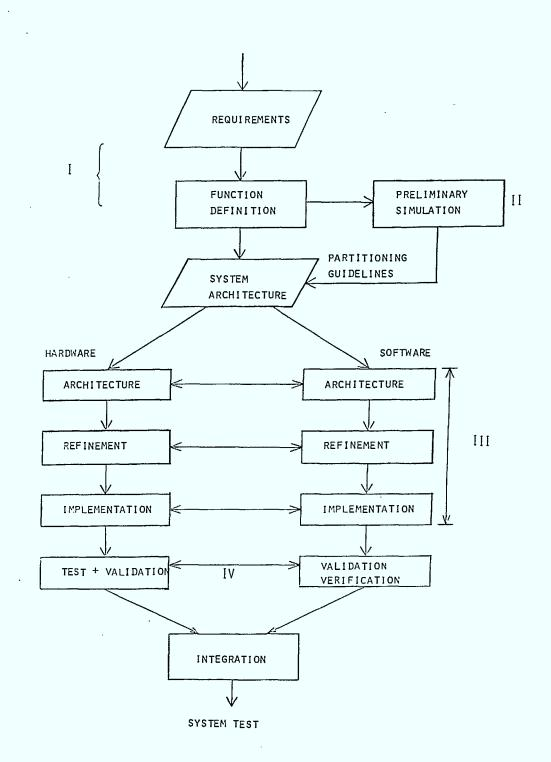
determine its correctness and its compatibility with the hardware. The second path involves determining the architecture of the hardware which is then refined in a series of top-down design steps. The hardware architecture is then simulated to determine its compatibility with the software. Following simulation, the hardware is implemented in a prototype which can be tested and validated. The hardware and software subsystems are then integrated and the resultant system is tested.
