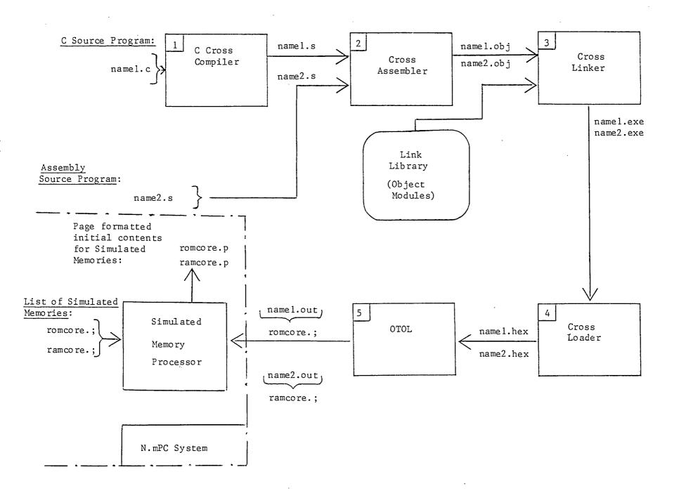
Figure 4-3 : Detailed Look at High-Level Software Development in N.mPc
