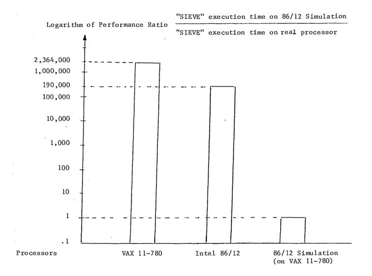
Performance Penalty due to Simulation using N.mPc
