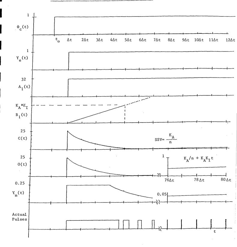
Theoretical Results from the SACL Algorithm(based on a continuous system)
