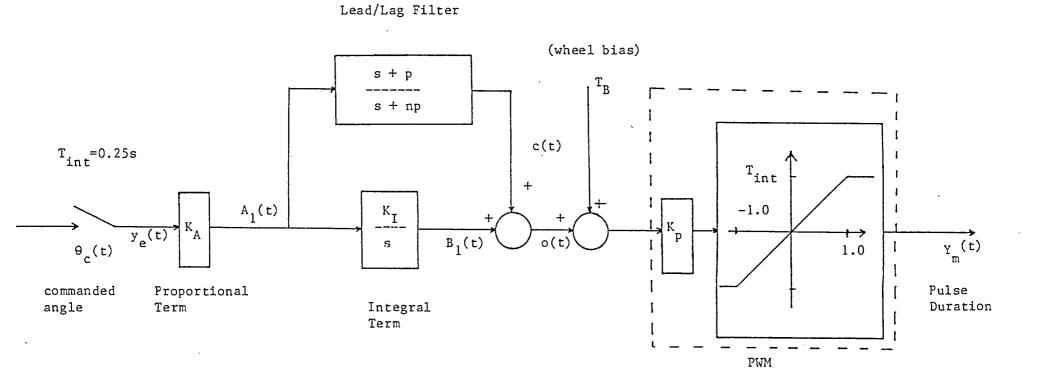
Input:  $\theta_{c}(t)$ , Commanded Angle Output:  $Y_{m}(t)$ , Pulse Duration
