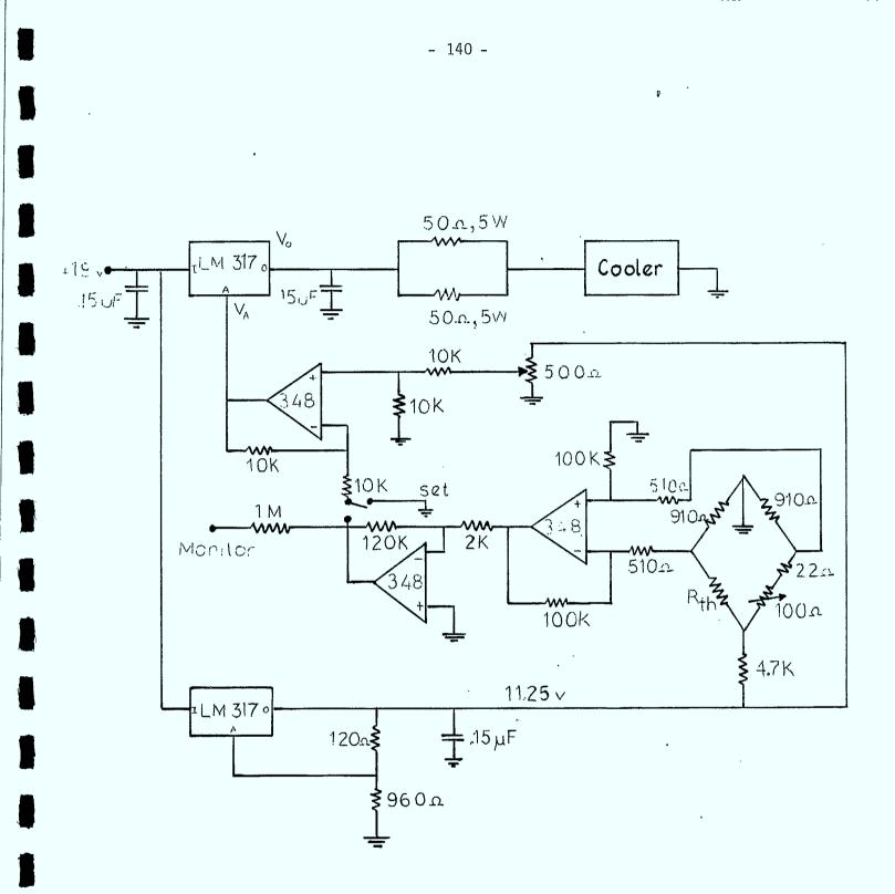
FIGURE 7.2.3: Temperature Control Circuit
