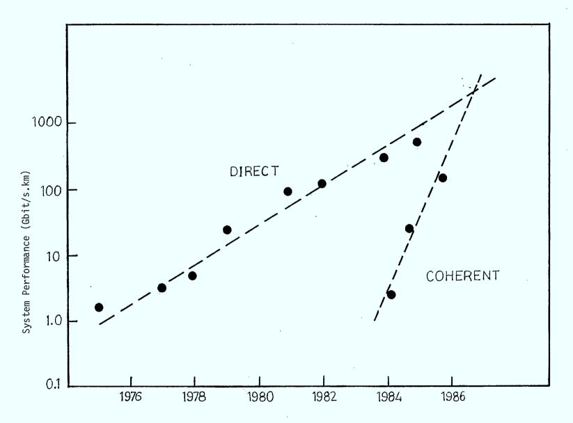
FIGURE 2.4.2: Progress in Coherent System Performance
