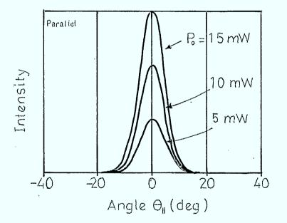
FIGURE 7.1.2: Typical Farfield Patterns for the HLP 1400 and HL8311E Lasers
