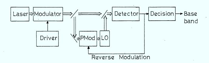
FIGURE 4.2.4: Basic Block Diagrams for a PSK Coherent Detection System
