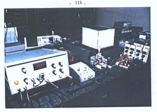
FIGURE 6.1.2(a): Experimental testbed. This photograph shows the transmitter in the foreground with bias circuitry in the box to the left of the laser assembly and the cooler control circuitry on the right. The local oscillator is housed in the white chamber. The detector is mounted on the three axis positioner immediately in front of the spectrum analyzer. The beamsplitter cube is immediately in front of the detector.
