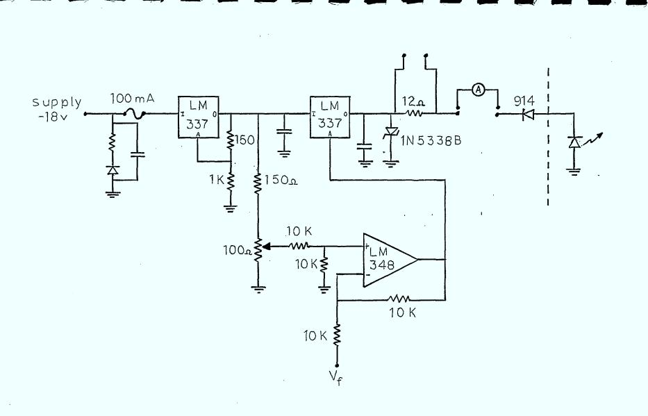
FIGURE 8.4.1: Local Oscillator Bias Circuit
