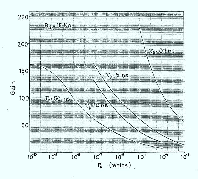
FIGURE 3.3.2: Optimum Gain as a Function of the Signal Power
