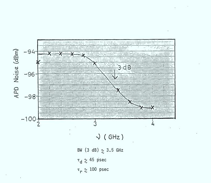
FIGURE 8.2.3: Antel APD Bandwidth Measurement
