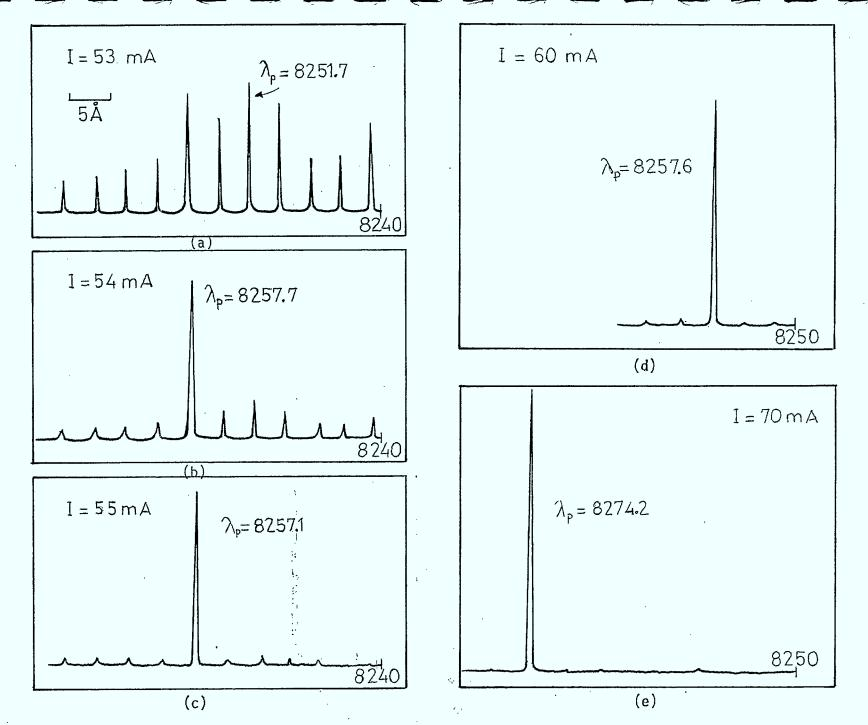
FIGURE 7.1.3: Continuous Wave (cw) Spectra for the HLP 1400
