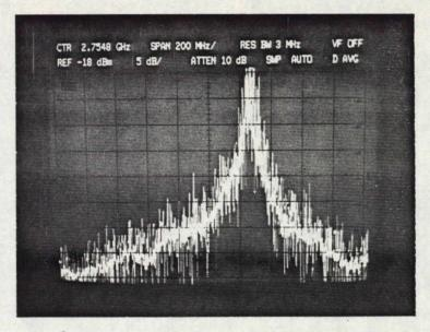
$P_{LO} = -9 \text{ dBm}$   $P_{Transmitter} = -10 \text{ dBm}$ Frequency Range:  $1.8 \rightarrow 3.8 \text{ GHz}$ Bandwidth: 3 MHzPeak Value: -14 dBmAmplification: 33 dB
