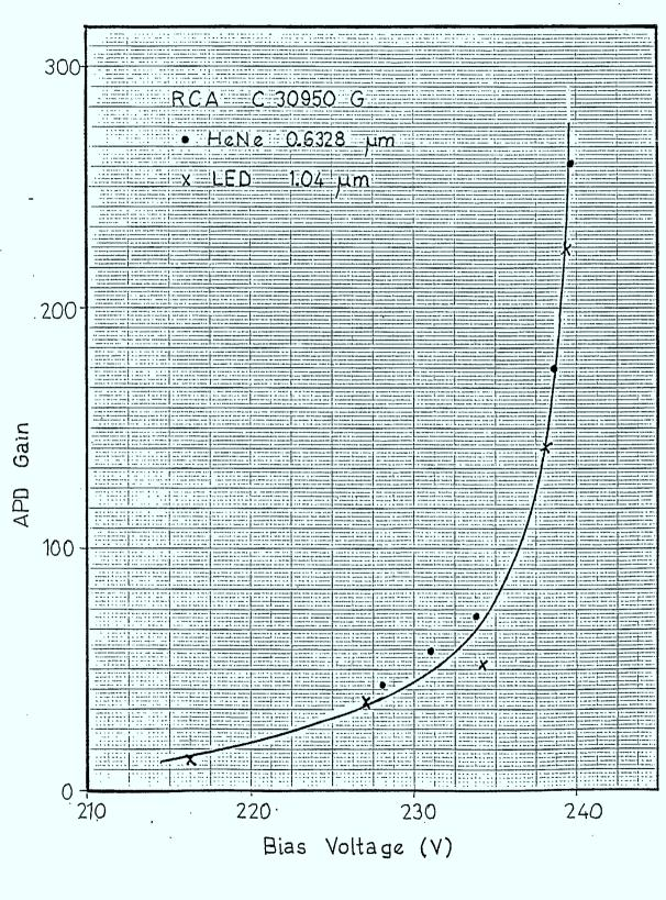
FIGURE 8.2.4: RCA APD Gain as a Function of the Bias Voltage
