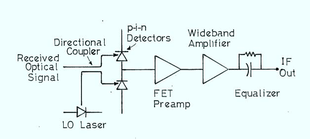
FIGURE 2.4.8: Dual Balanced Detector Configuration Used in the 1 Gbit/s DPSK Coherent Experiment
