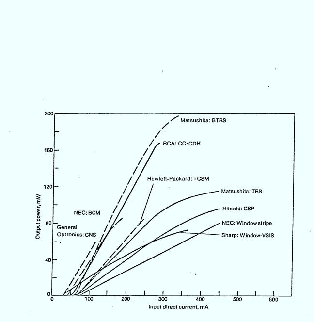
FIGURE 2.4.4: Best Published Results of Light-Current Characteristics for GaAlAs Devices of the Structures Shown in Figure 2.4.3. future.
