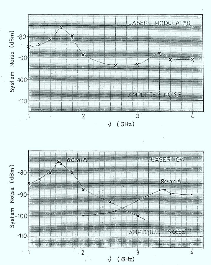
FIGURE 9.1.5: Comparison Between System Noise for Pulse and cw Laser Operation
