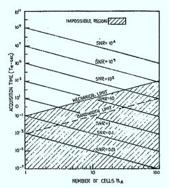
Fig. 2. Effective scan period versus number of cells  $n_A$  for various SNR.
