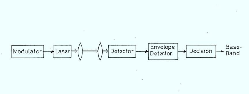
FIGURE 4.1.1: Basic Block Diagram for an Intensity Modulated/Direct Detection System
