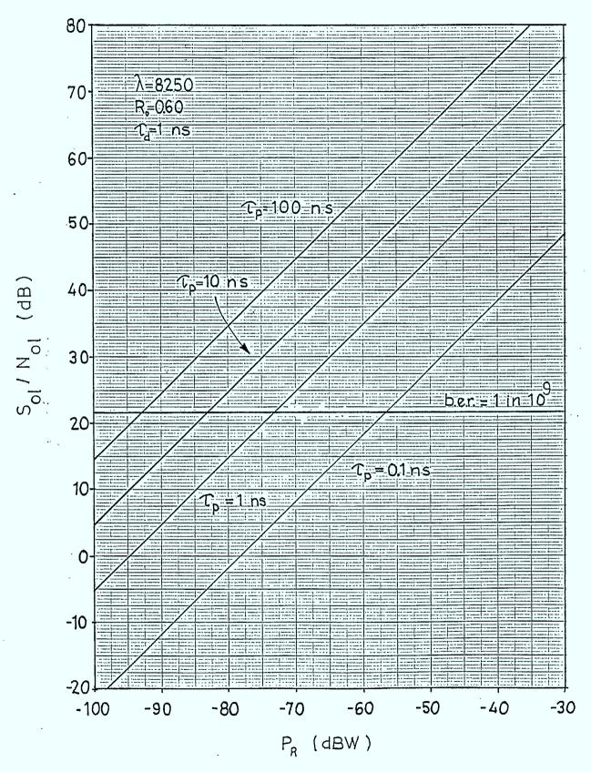
FIGURE 3.4.5: Optimum Signal to Noise Ratio as a Function of the Received Power
