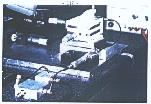
FIGURE 6.1.2(c) This photograph shows the elements of the frequency discriminator. Following the detector comes the pre-amp, the filter, the power splitter and finally the balanced mixer. The coaxial delay line between the splitter and the mixer can be seen to the left of these components.
