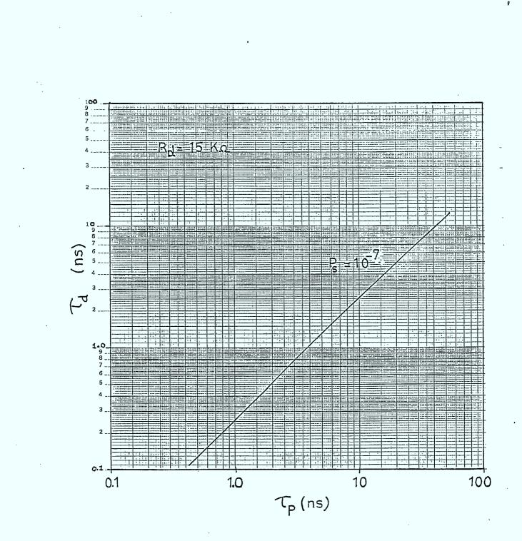
FIGURE 3.3.4: Optimum Detector Time Constant as a Function of  $\tau_{\rm p}$
