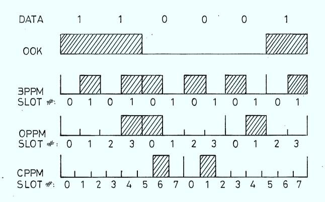
FIGURE 4.1.2: Bit Streams in OOK and PPM Modulation Schemes
