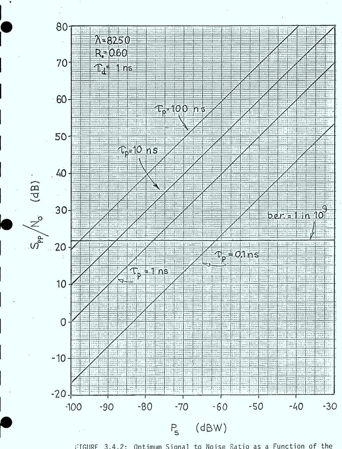
FIGURE 3.4.2: Optimum Signal to Noise Ratio as a Function of the Received Power
