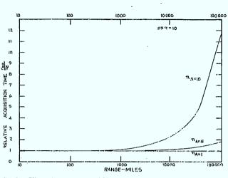
Fig. 3. Effect of range on acquisition time.
