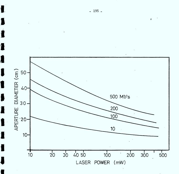
FIGURE 9.4.1: Aperture Size Dependance on ISL Distance
