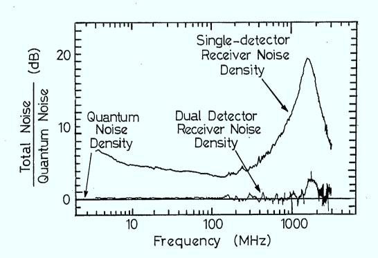
FIGURE 2.4.7: Schematic of a Dual Balanced Detector Receiver and Measured Noise Performance
