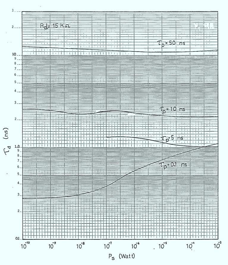
FIGURE 3.3.3: Optimum Detector Time Constant as a Function of the Signal Power
