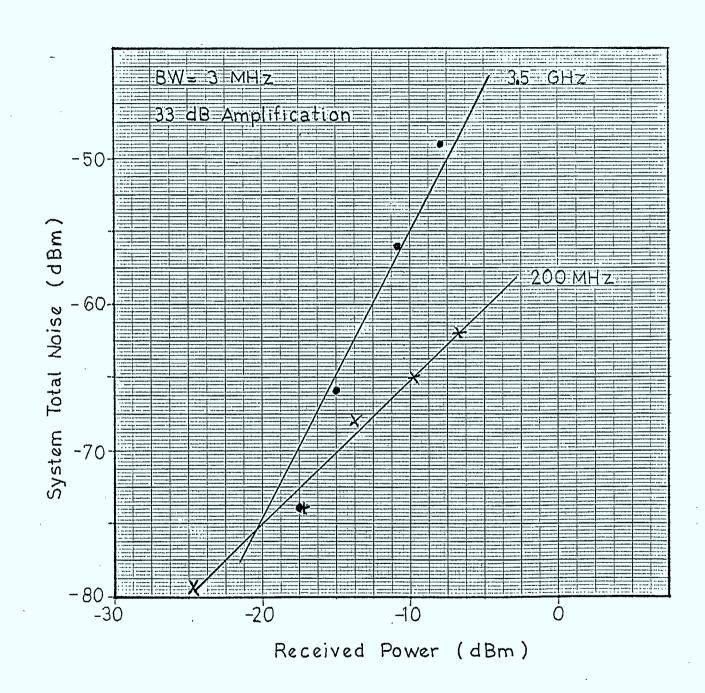
FIGURE 9.1.6: System Noise Variation as a Function of the Received Power
