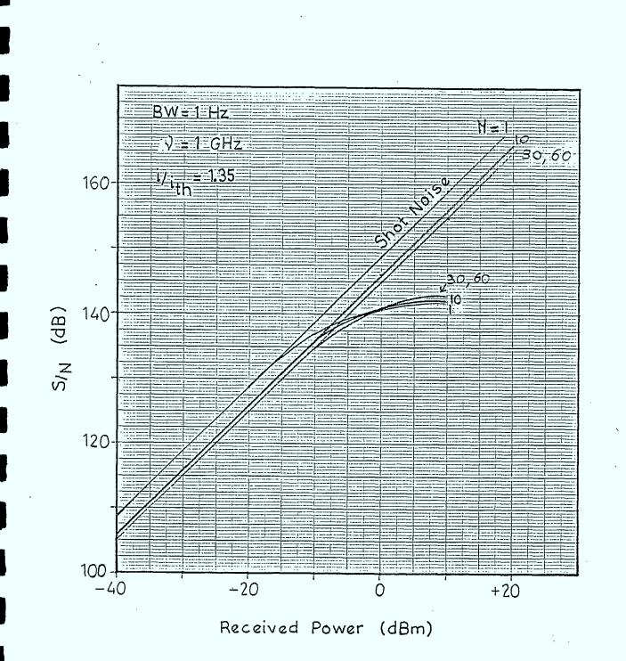
FIGURE 9.1.7: Signal to Noise Ratio as a Function of the Received Power for Various APD Gain Values
