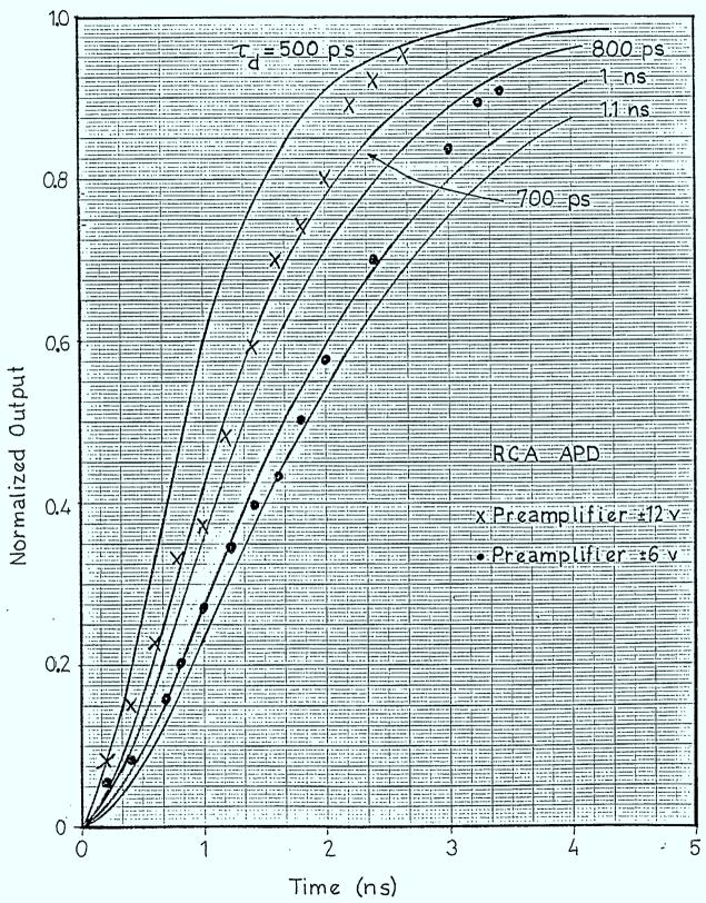
FIGURE 8.2.2: RCA APD Time Response Measurement
