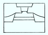
Self-aligned Strip Buried Heterostructure (SSBH)
