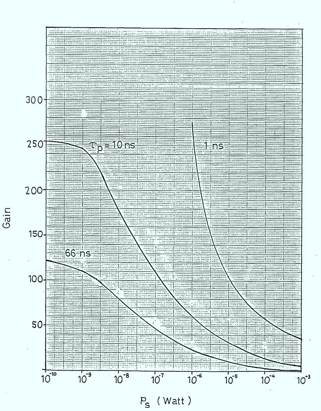
FIGURE 3.3.6: Optimum Gain as a Function of the Signal Power
