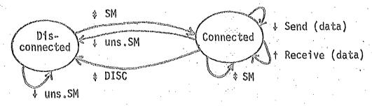
Note: This diagram represents an abstraction of the operation of the HDLC protocol at the given station.
