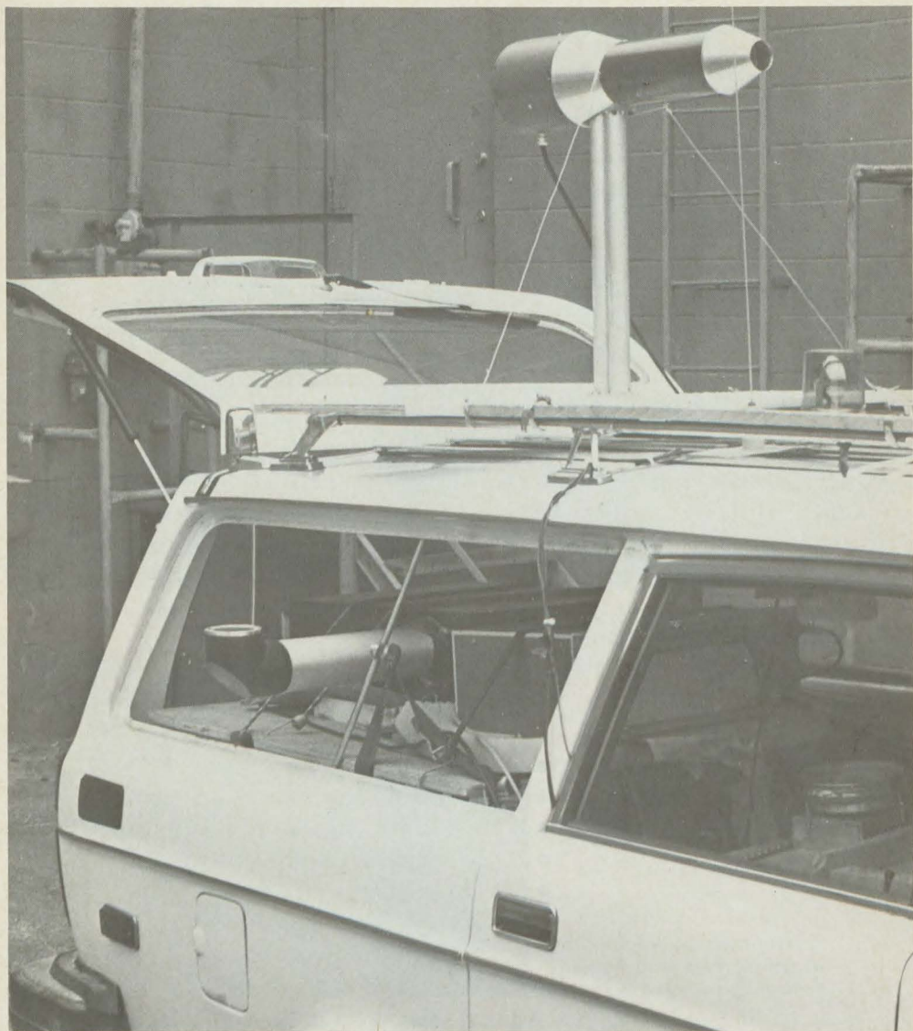
Air intake for fast response mobile \text{SO}_2 ambient monitor, mounted atop automobile with PLUMETRACKER.
