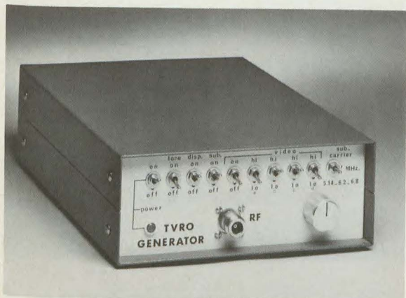
Electrohome TVRO generator of test signals to verify functionality of satellite receiver with 1 GHz and 4 GHz outputs.
