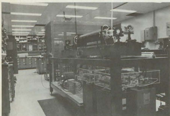
An aperture injection-locked atomic iodine laser for use in plasma physics experiments.
