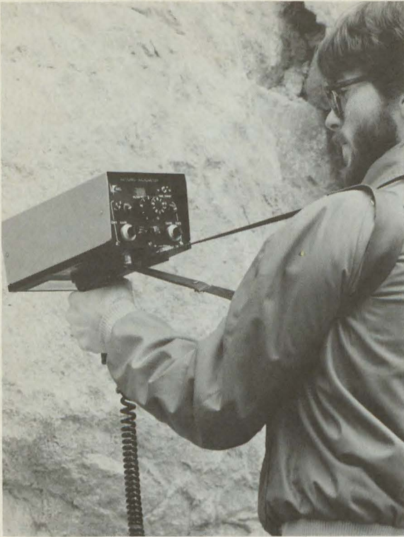
Barringer hand-held Ratioing Radiometer to conduct ground truthing and improve interpretation of LANDSAT or SPOT imagery.
