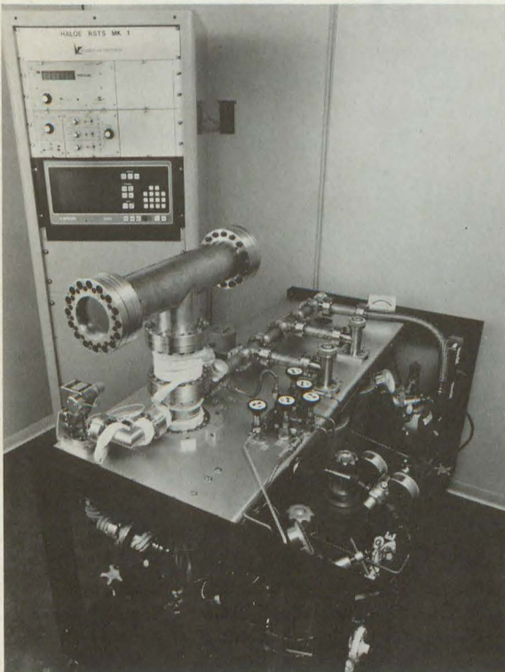
Barringer ultra high vacuum pumping station and calibration cell ground support equipment for HALOE Project.
