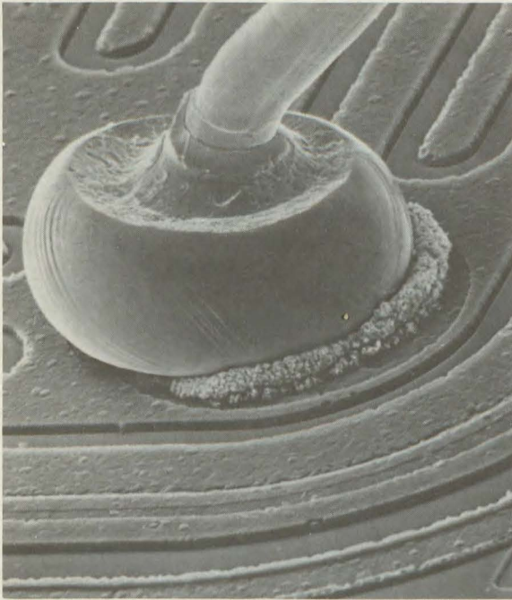
Scanning electron micrograph of intermetallics at gold wire 0.0012 diameter bond of a transistor rejected for use on the NASA space shuttle.
