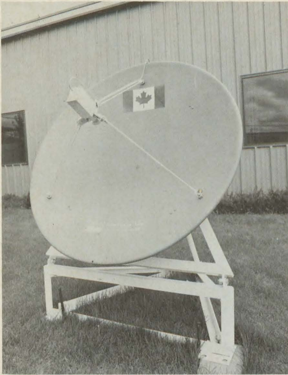
SED small diameter satellite communications direct broadcast 12 GHz terminal.
