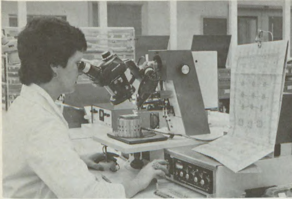
CMC manufacturing operation for hybrid microcircuits for space-related and other applications.
