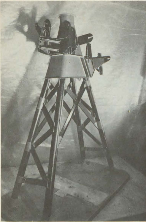
Lightweight Boeing graphite epoxy and kevlar tower support structure for use on a communications satellite.
