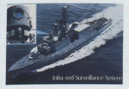
Shipboard infra-red surveillance system by Spar.
