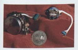
Litton-made accelerometers for inertial navigation systems.
