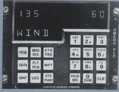
CMC's line of Omega/VLF systems features the CMA-771 Alpha, with a solid-state alphanumeric control/display to communicate with the operator, a capacity for 500 stored way-points, and an interface to Nav Data banks such as the Vandling NDB-2. The CMA-771 readily encompasses future software advances, since the computer-entry mode allows for a wide variety of applications.
