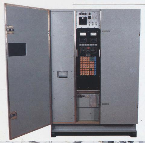
The AN/SPS-503 is an E/F (S) band, shipborne Air Search Radar which can be used in severe ECM and sea clutter environments. Frequency agility, pulse compression and advanced signal processing techniques provide superior performance in a compact and lightweight system. It is ideally suited for fitting to ships as small as 300 tonnes.
