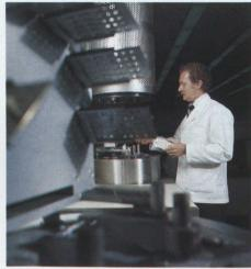
Vacuum evaporation machines deposit pure silver or aluminum electrodes on crystal blanks.
