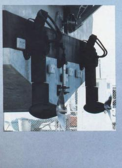
Grumman Aerospace Corporation patrol hydrofoils use Maritime Industries units for emergency propulsion and manoeuvring in confined areas
