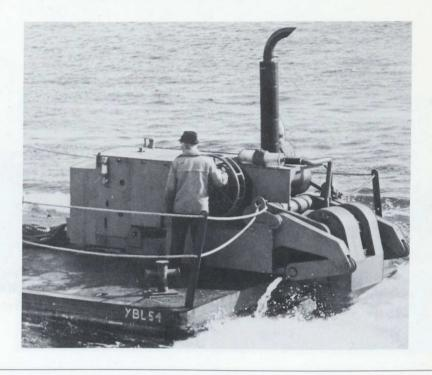
The concept of packaging all propulsion, steering and fuel tanks into a portable bolt-on-deck unit is beginning to make a lot of economic sense to more budget-restricted work barge and ferry fleet operators. And they can thank Maritime Industries Limited for the idea.
