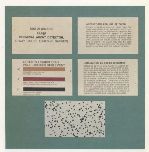
action, if coloured spots or streaks appear on the paper, the troops immediately don their protective masks. The type of agent may then be determined by comparing the colour of the spots or streaks on the paper with the colour chart.
