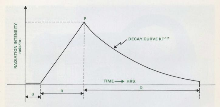
d - delay time - time from start until first indication of fallout R - Rise time - time from start of fallout indication to time peak intensity is reached P - Peak value - maximum intensity of radiation D - Decay time — period from peak value to the time the program is automatically terminated by the Simulator
