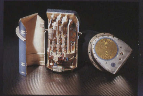
An early prototype 'FXR', MM-Wave Frequency Extension for radar warning receivers . . .
