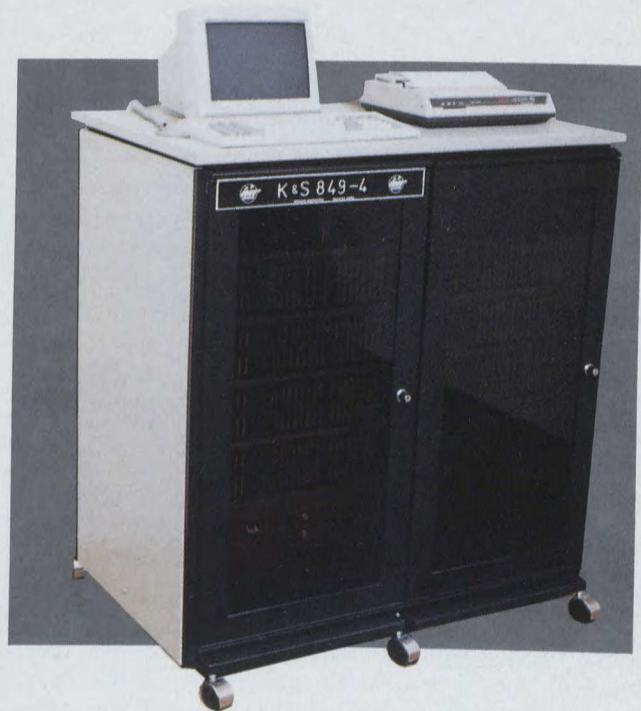
IMP Aerospace Manufacturing Plant and new generation automatic test equipment designed and manufactured by IMP for use on electronic wire assemblies and electronic systems
