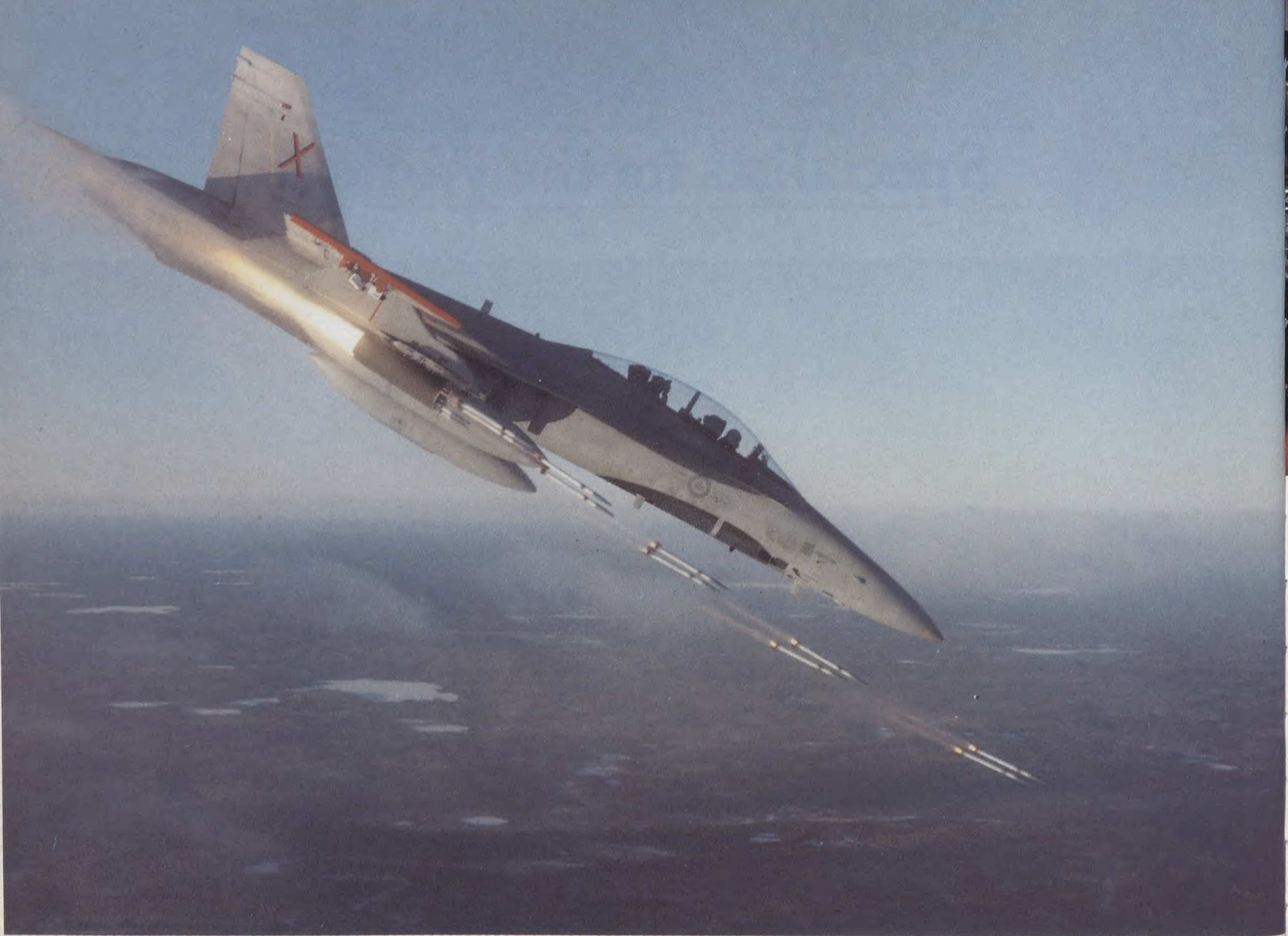
A Canadian Forces' dual CF-18 firing CRV-7 high velocity rockets from Bristol Aerospace.
