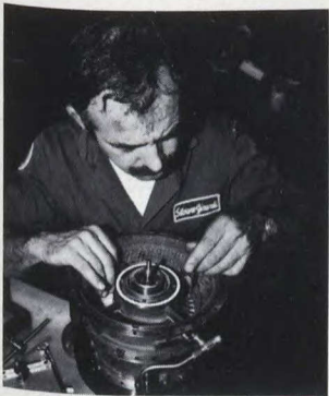
Technicians building a C30 turbine module (left) and balancing a CT58 rotor (right). Canadian builds its engines to very tight tolerances as part of its efforts to improve unit reliability.
