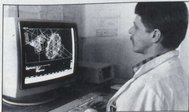
5779-22 - C-130 component displayed on a Sun 3/60 CAD/CAM station
