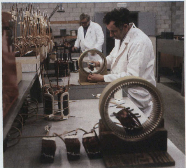
Electrical Component Rewind Facilities.
