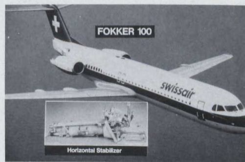
Fokker 100 horizontal stabilizer actuation system, designed and manufactured by Menasco in Oakville, Ontario.
