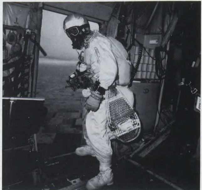
Irvin Military Parachuting Equipment: FF-2 Hitefinder Automatic Parachute Release mechanism, PA-100 Military Parachutist Altimeter and CT-3 High Glide, Tactical Ram Air Parachute System for High Altitude, High Opening (H.A.H.O.) military standoff, parachuting operations.
