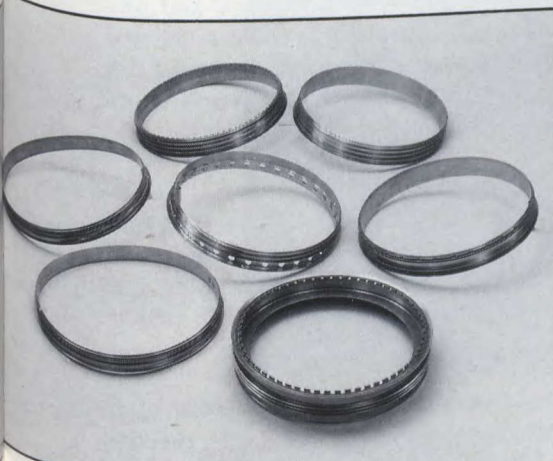
F100 titanium and waspalloy compressor air seals
