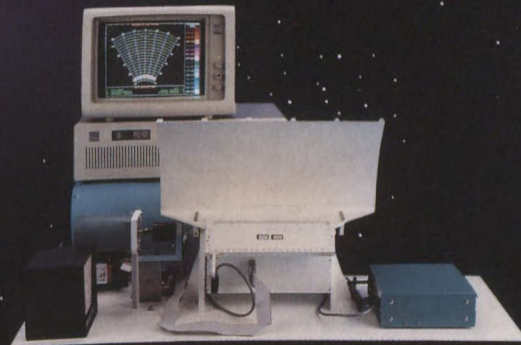
An Electrically Scanning Millimetre-wave Radiometer for ice detection.
