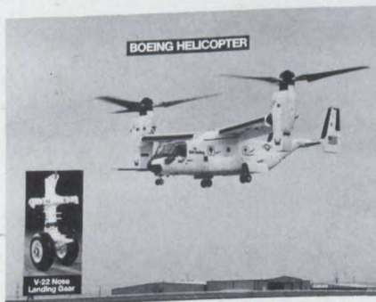
Menasco designed and built the nose landing gear, retract actuators and drag brace systems on the new Bell Boeing V-22 Osprey; seen here on its maiden flight.
