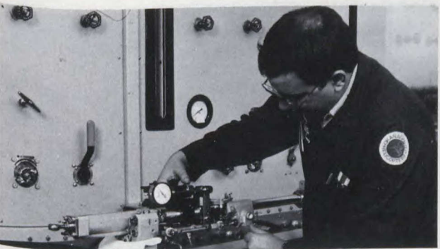
ACCESSORY SHOP - A hydraulic servo being tested after overhaul on Canadian's hydraulic test unit. The accessory shop overhauls a variety of hydraulic, electrical and electromechanical accessories.
