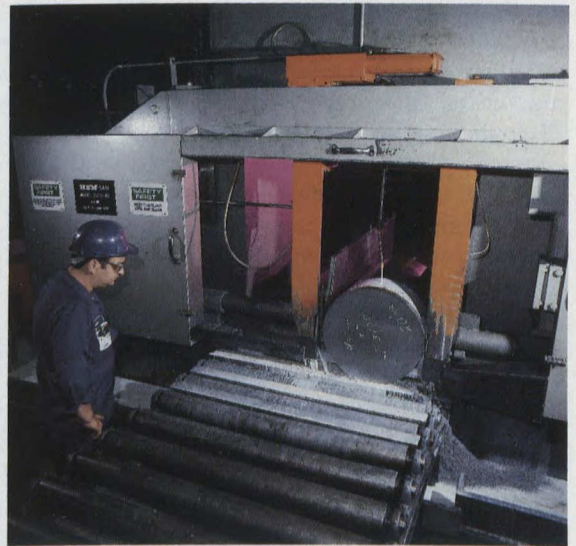
Hem saw cuts disc from alloy steel bar.
