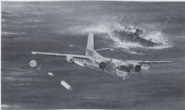
Light Weight Survival Kit, Air Droppable (L.W. SKAD): a completely self-contained, wing-mounted sea rescue system that is automatically sequenced to deploy, deliver and inflate two 6-man life rafts, and accompanying survival equipment in close proximity to endangered personnel.
