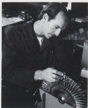
Technicians building a C30 turbine module (left) and balancing a CT58 rotor (right). Canadian builds its engines to very tight tolerances as part of its efforts to improve unit reliability.
