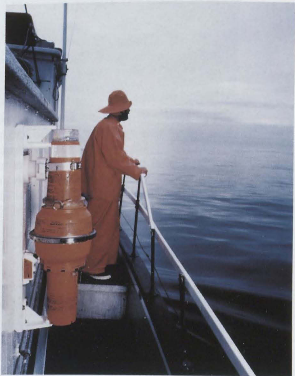
406 MHz satellite rescue beacon (EPIRB) — first of a family of emergency communications products designed by MPR Teltech. (Photo courtesy of Alden Electronics Inc. of Westborough, MA).
