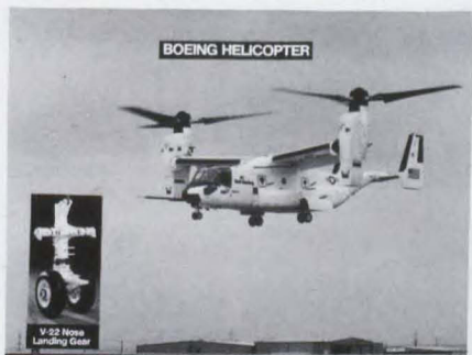
Menasco designed and built the nose landing gear, retract actuators and drag brace systems on the new Bell Boeing V-22 Osprey; seen on its maiden flight.
