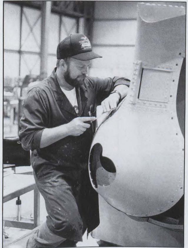
This capability enables skilled repairs to be made on aircraft components such as this helicopter fuel tank
