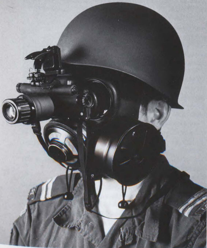
Light-weight, low cost night vision goggles utilize image intensification technology.
