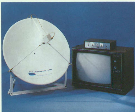
The equipment pictured here is all the Canadian homeowner of the future (as early as the mid-80's) would need to receive high-quality color TV direct from satellites. At left is a 60 cm parabolic dish antenna with a tiny outdoor electronics package mounted opposite its centre. This antenna unit feeds satellite signals to the small receiver/converter unit atop the standard TV set.
