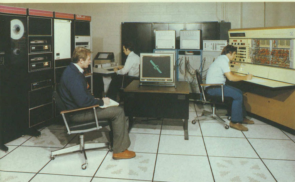
This hybrid computer at the Communications Research Centre combines digital and analog computing methods and is used in the design and simulation of attitude control systems for spacecraft.
