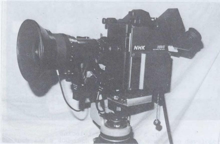
Fig. 4 Portable camera for HDTV
