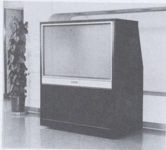
Fig.13 55-inch rear projection display.
