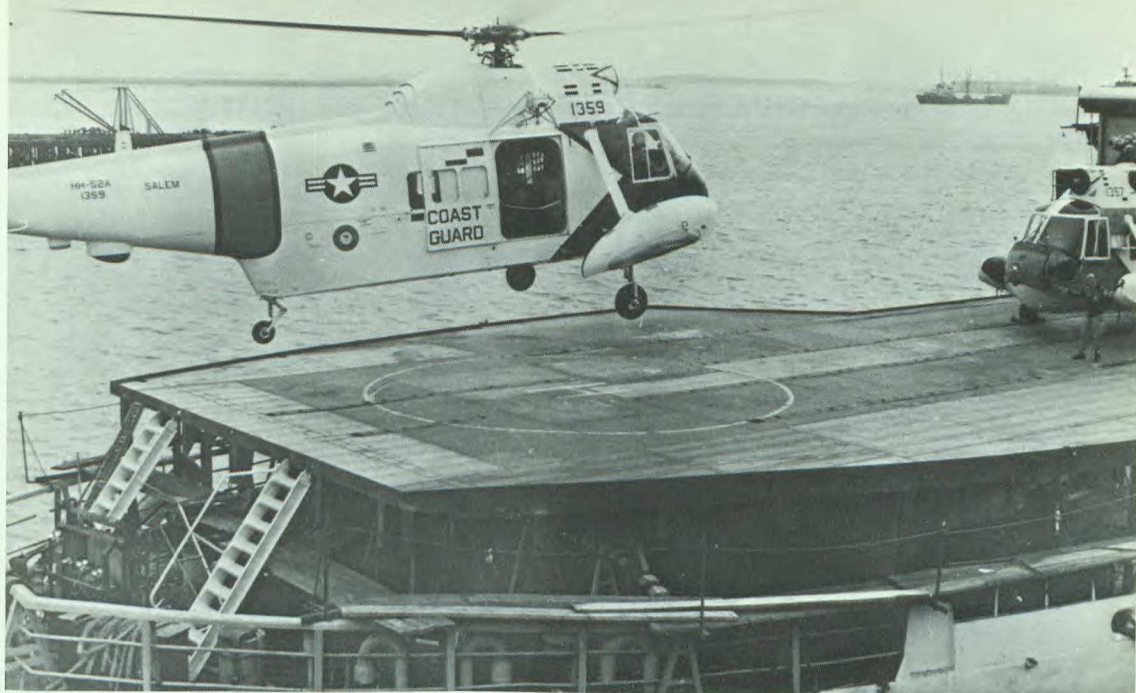
Sikorsky HH-52A landing on U.S.C.G.C. "Eastwind" with the hangar retracted. Retracted length 18'9½" (5.7m).
