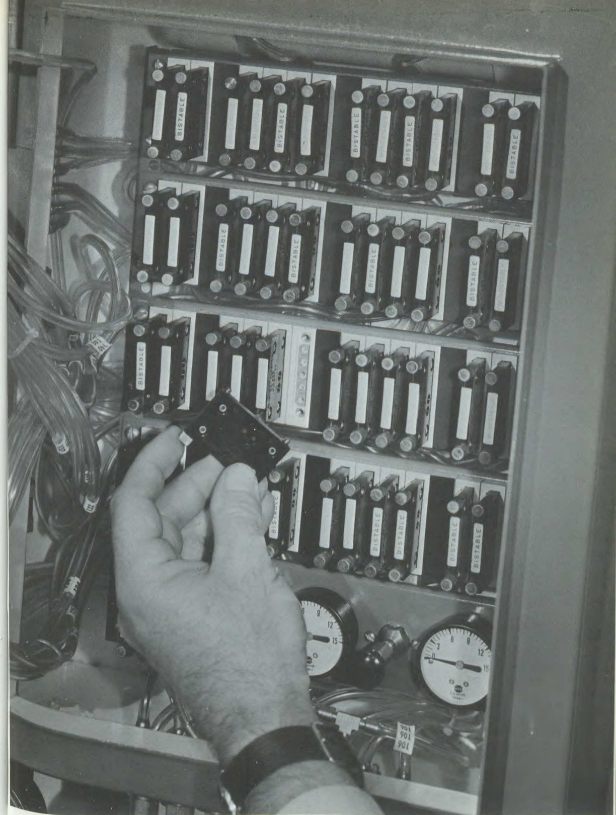
An "Edgemount" fluidic industrial sequencer control panel, demonstrating the easy replacement of elements and/or circuit modification now made possible with Aviation Electric's new modular design concept. All elements are plugged in to standard sockets, thus eliminating the tangle of interconnecting tubing usually associated with fluidic circuits.
