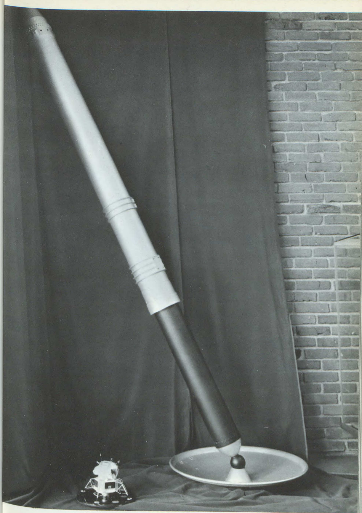
A LEM leg with a representative landing pad at the base. A model LEM is shown in the left foreground.
