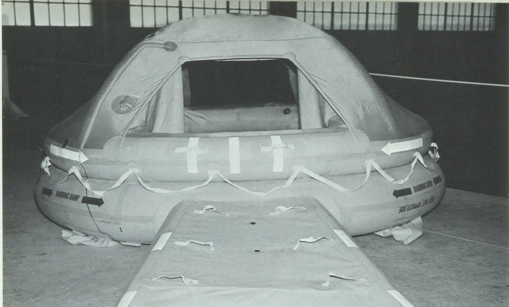
This version of a 10 man raft differs from the one described in the article but serves to point out the variety of original designs offered by TUL. The boarding ramp may be seen together with the opened primary and secondary closure curtains. The water activated battery cell and emergency light are at the left of the canopy opening.
