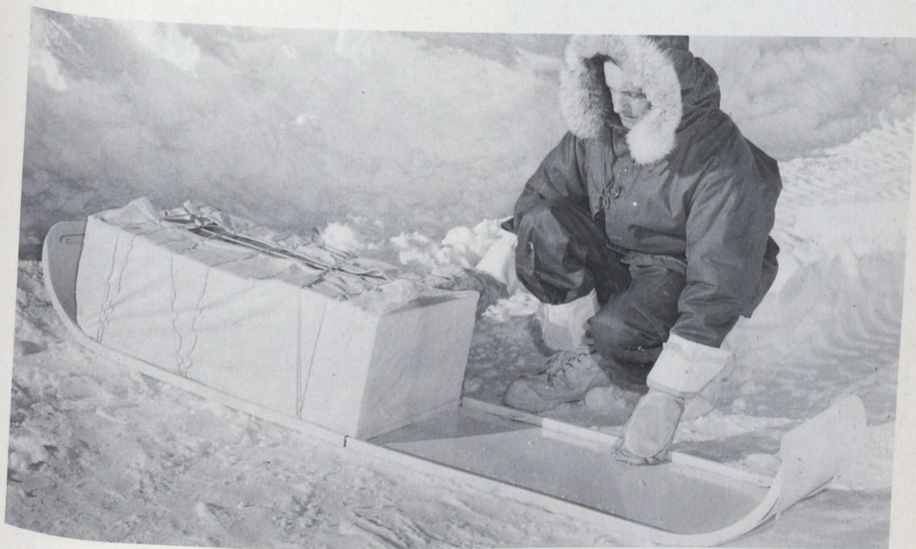
Two 45.4 kg Toboggans being joined to make one larger carrier.
