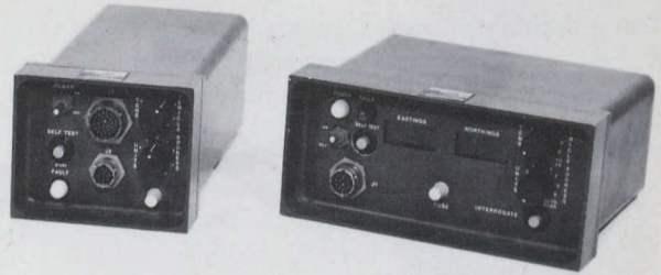
PITS units: vehicles Transponder at left and command post interrogator
