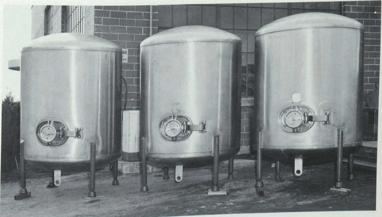
Stainless steel vessels with inside welds finished to #4 polish to meet strict sanitary code requirements. Constructed of type 316 stainless steel, they are 2.4 m (8 ft) high with a 1.8 m (6 ft) diameter.
