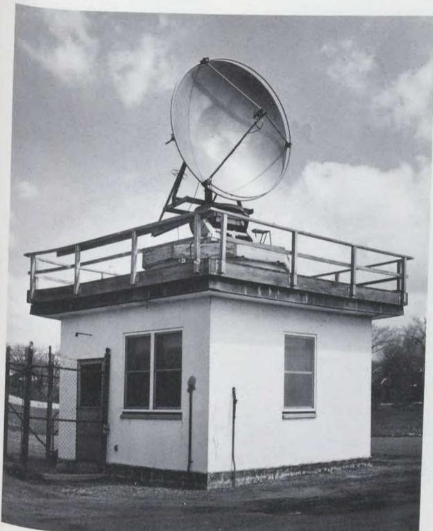
Radiation pattern measurements of a parabolic reflector antenna.
