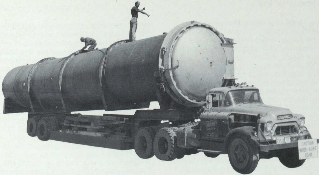
A 16.7 x 2.4 m (55 x 8 ft) autoclave constructed to code UW12A and fabricated from A212B firebox plate with a working pressure of 7 kg/cm 2 (100 PSI).
