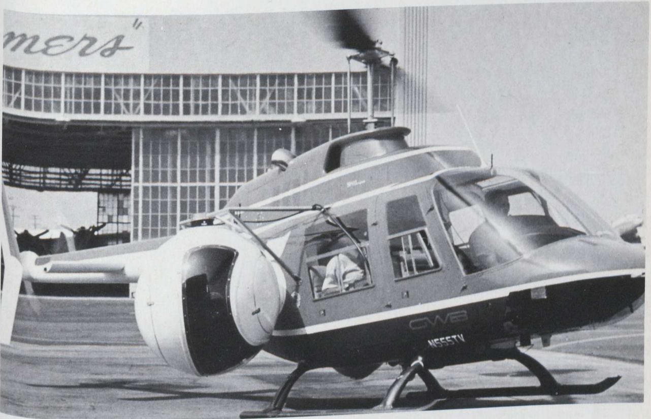
HC-32 WESSCAM Mount fitted to a Jet Bell Ranger.
