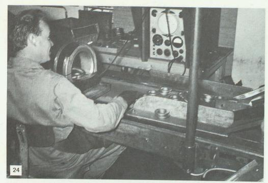
Magnetic testing of flanged rings with readout on oscilloscope.
