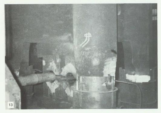
Finish forging of an axle on a pulldown type hydraulic press.
