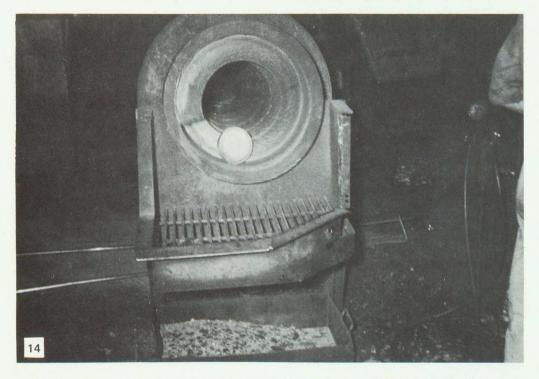
Circular billet seen at discharge end of an inclined internal spiral conveyor. Note a pan filled with scale removed as the billet rotates in the spiral conveyor.
