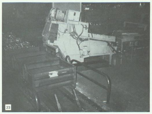
Demagnetizer conveyor delivers parts to tote boxes after crack inspection. Note automatic shifter for tote boxes after filling.
