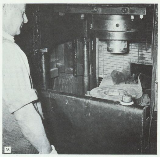
Cold forged part, seen on front press guard, is made in one stroke on a cold forging press at English Steel.
