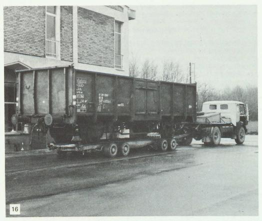
Railway gondola car at the Carlo Raimondi plant in Italy, after being transported to the weigh scale by a highway tractor trailer.
