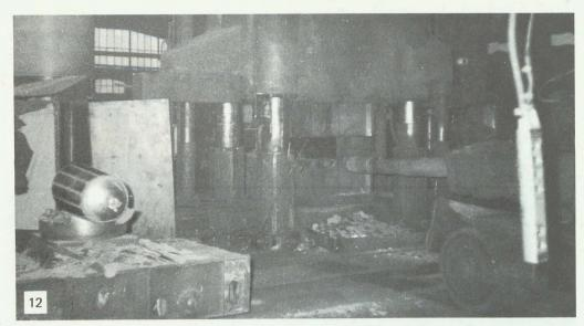
Manipulator and hydraulic press just completing rough forging of an axle at Italsider.
