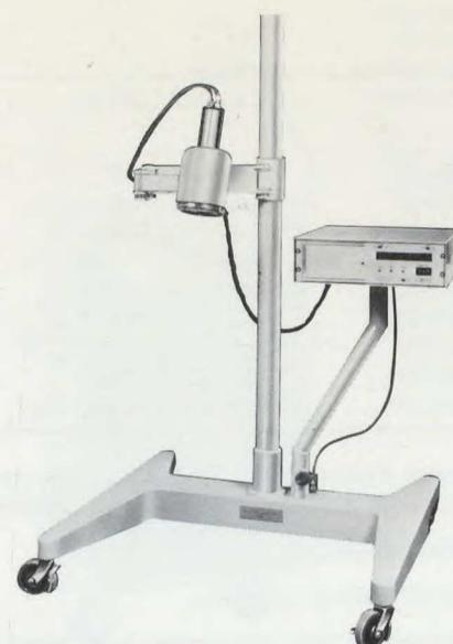
*701DS single channel system with 611D Scaler-Spectrometer*
