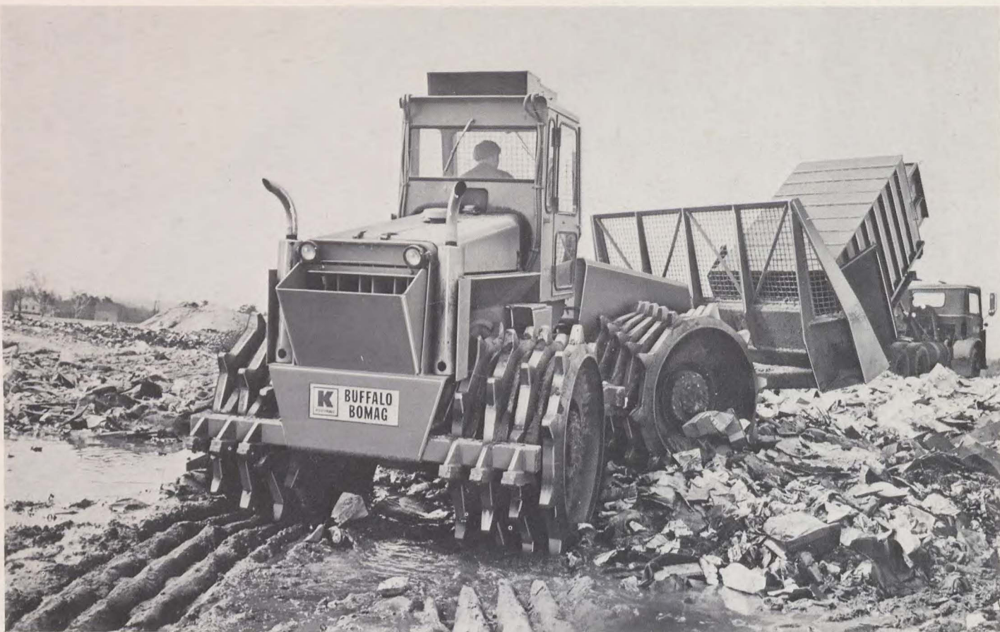
The Buffalo-Bomag's continuous full-width wheel coverage makes every pass count.
