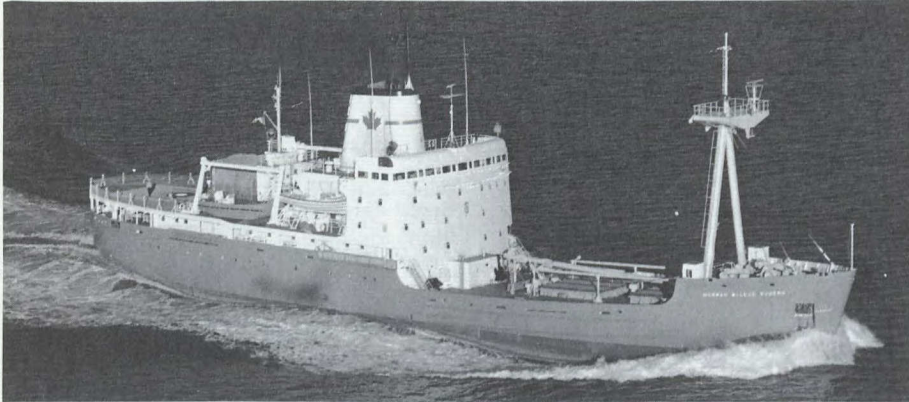
The world's first gas turbine icebreaker, the "Norman McLeod Rogers", is powered by twin Westinghouse engines.
