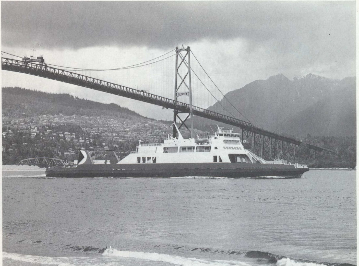
Power and efficiency are combined with a pleasing appearance in the "Carrier Princess", which recently went into service as a trailer/rail car ferry between Vancouver and Schwartz Bay, British Columbia. Designed by Talbot, Jackson & Associates, the ship has an overall length of 380 ft. (116 m) and can transport 50 trailers or 30 rail cars.
