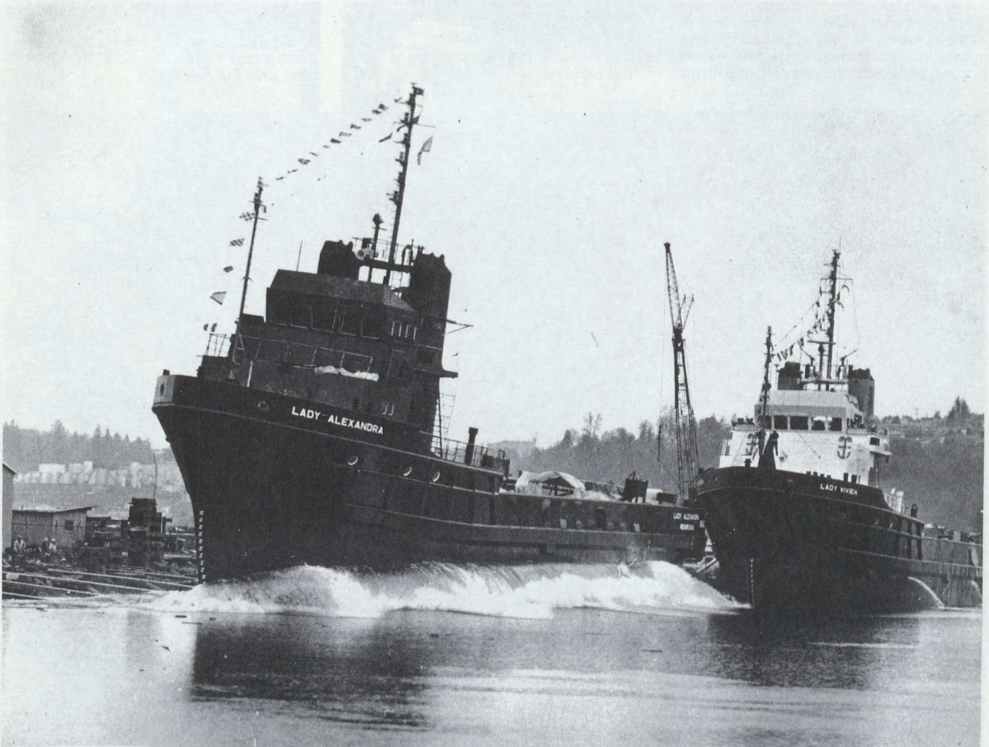
The "Lady Alexandra" slips into the water from the side-launching berth at Allied Shipbuilders.
