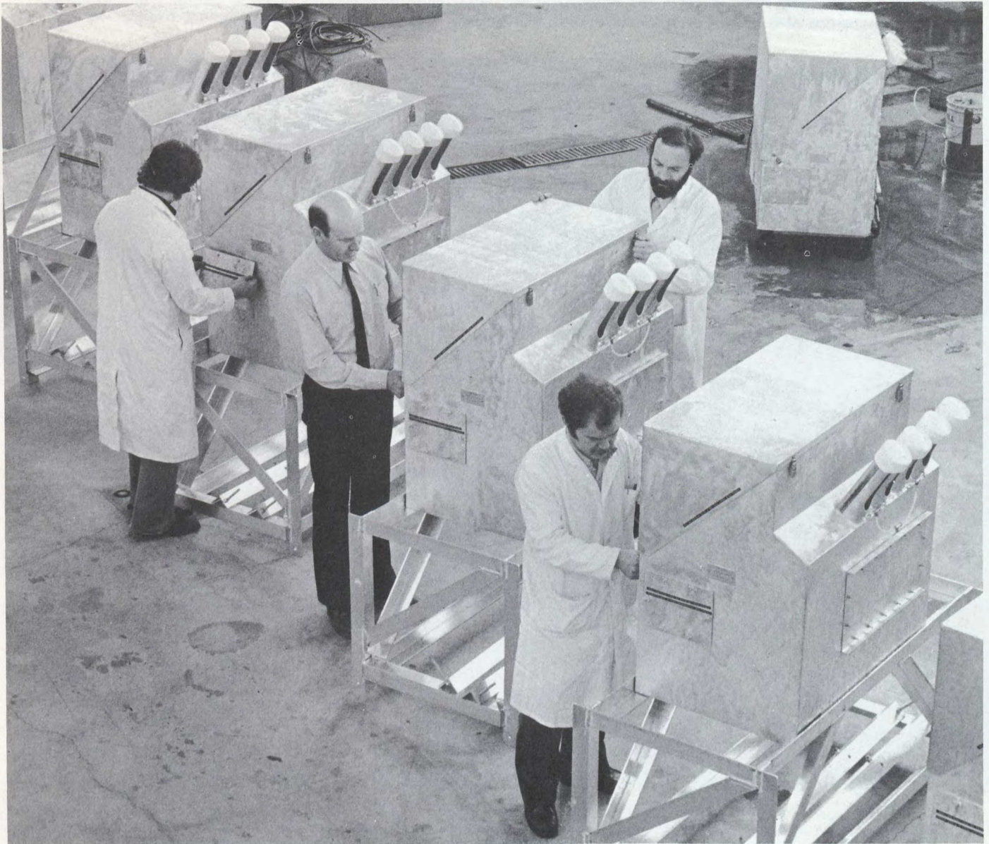
Techwest Enterprises staff examine a shipment of herring sex sorters destined for the B.C. roe herring industry.
