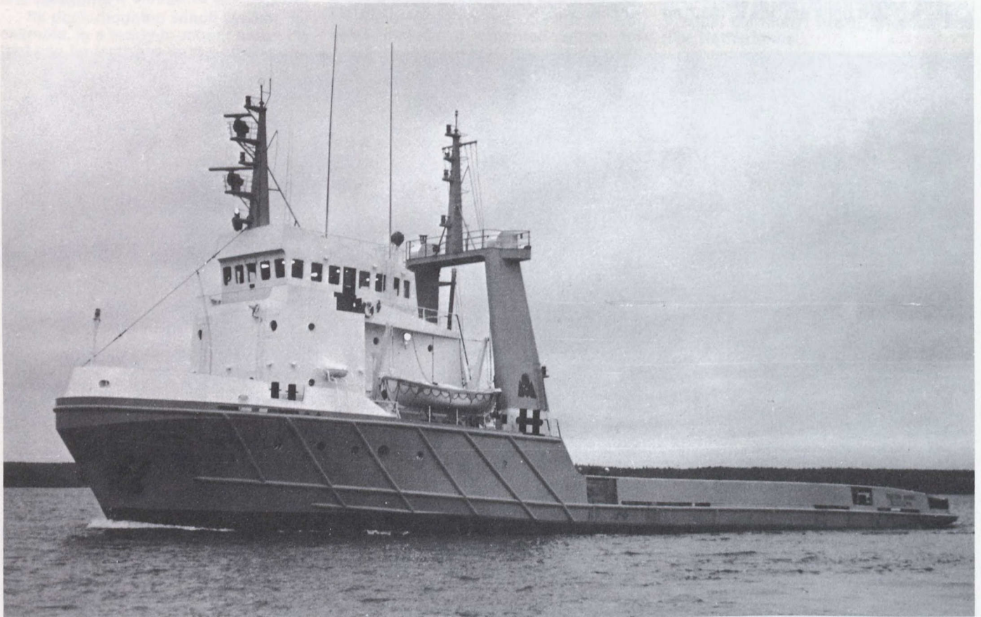
Built by Ferguson Industries Limited to Lloyds Ice Class II specifications, this rugged tug/supply vessel is designed for use in the Atlantic, North Sea and other northern waters.
