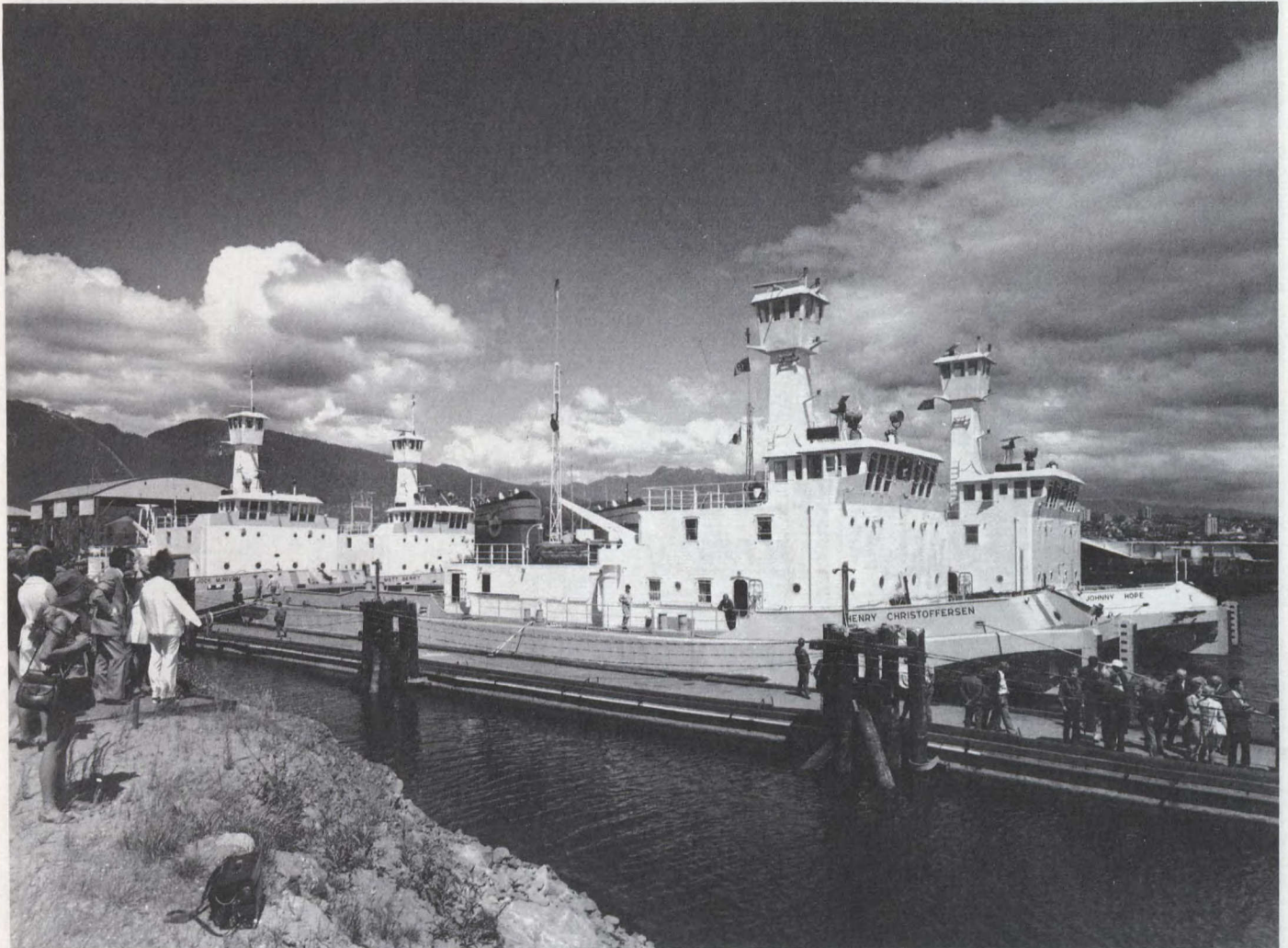
Robert Allan Ltd. designed these four quadruple screw, shallow-draft tugs for use in the Mackenzie River/Beaufort Sea areas by Northern Transportation Ltd. The vessels measure 155 ft. (47.3 m) o.a., 52 ft. (15.85 m) in breadth, 10 ft. (3.05 m) in depth and have a maximum loaded draft of 4 ft. (1.22 m). Two of the tugs have nozzle propulsion and two feature open tunnel propulsion. They can handle barge trains of 9,000 tons (8,916 metric tons).
