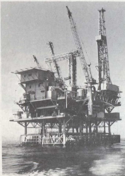
Westburne Petroleum Services Ltd. specifically designed this slant hole drilling rig for offshore petroleum exploration.
