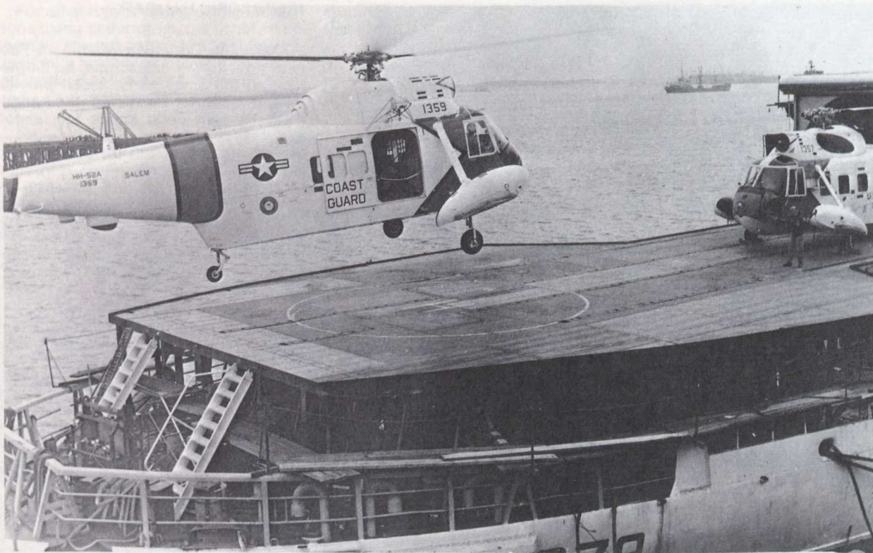
Landing Sikorsky HH-52A helicopters on United States Coast Guard Cutter "Eastwind" with the hangar retracted to a length of 18 ft. 9½ in. (5.79 m).
