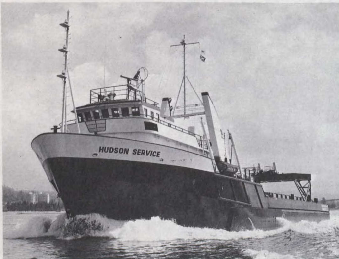
This offshore supply vessel, M.V. "Hudson Service," is equipped with an ANKER controllable pitch propeller system from General Propulsion Systems Ltd. The vessel has 3,500 hp per shaft.
