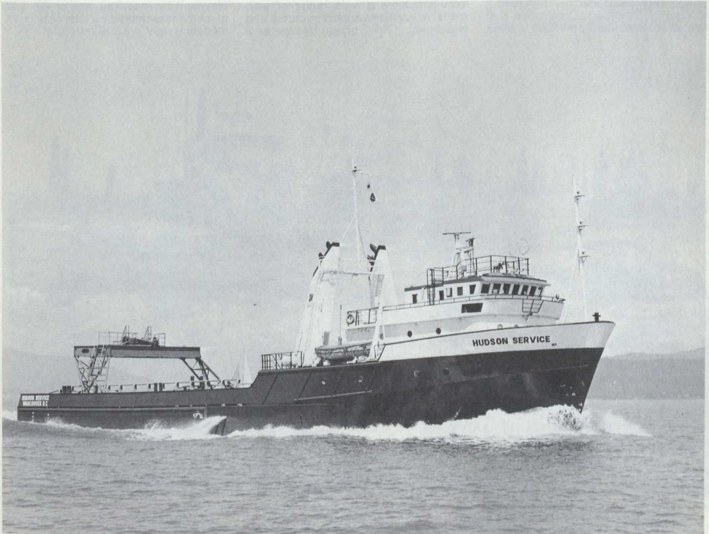
Built by Bel-Aire Shipyard Ltd., the 185-foot (56.39 m) "Hudson Service" plows through the waters of Vancouver harbour during trial runs. The ice-strengthened offshore supply vessel is powered by four General Motors EMD diesel engines producing 6,560 hp.
