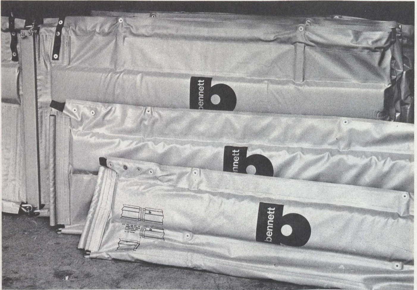
Inshore oil booms manufactured by Bennett have rapid deployment capability and fully integrated construction, are easy to clean and are compact for ease of storage. Boom sizes are 18 in. (45 cm), 24 in. (60 cm) and 36 in. (90 cm). Freeboard measurements are 6 in. (15 cm), 8 in. (20 cm) and 12 in. (30 cm) with drafts of 12 in. (30 cm), 16 in. (40 cm) and 24 in. (60 cm).
