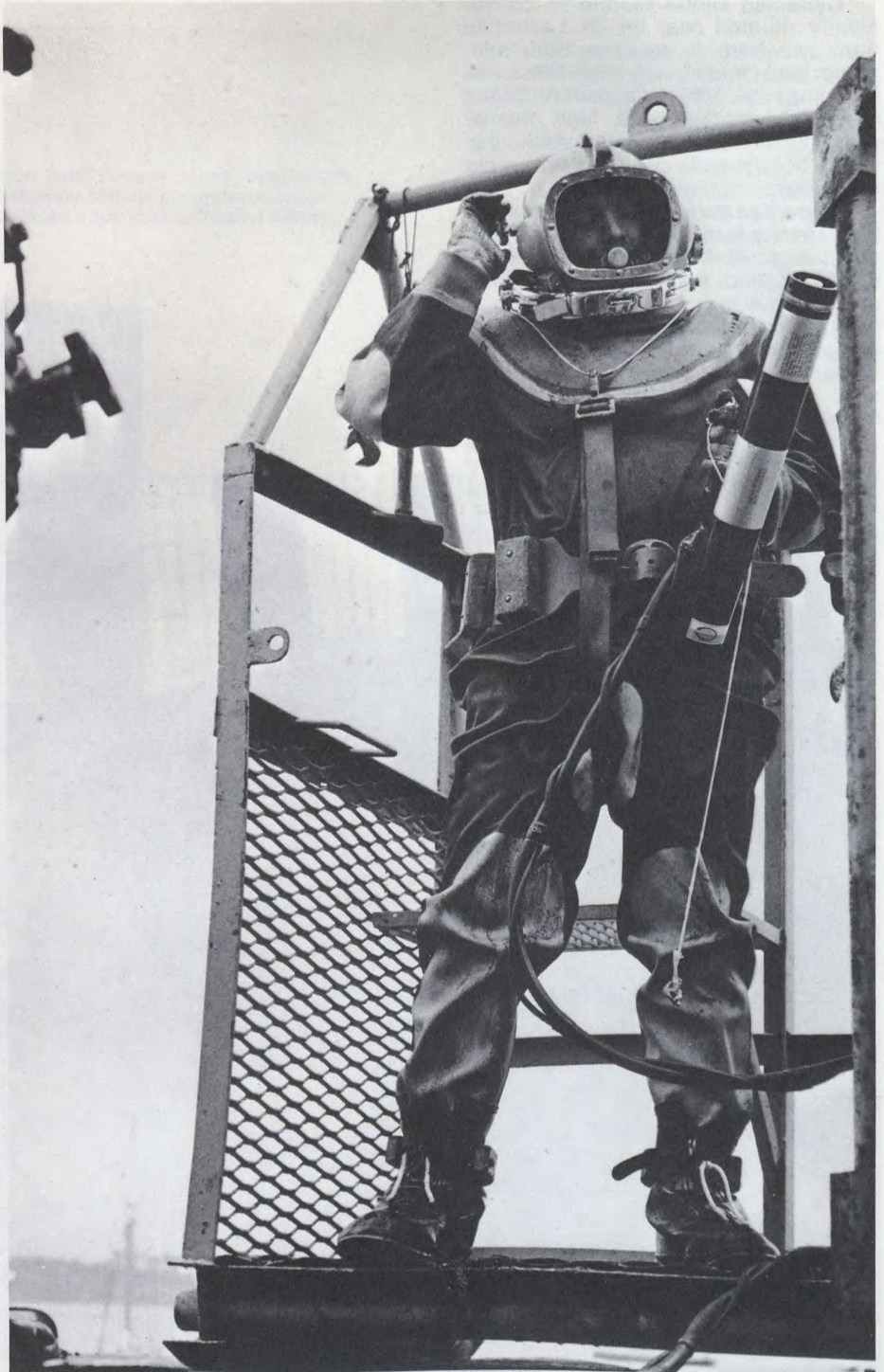
Preparing for deep descent, a Can-Dive Services diver adjusts his helium/oxygen supply. Can-Dive provided Canadian industry with the first offshore petroleum support service using the HeO 2 deep diving technique.
