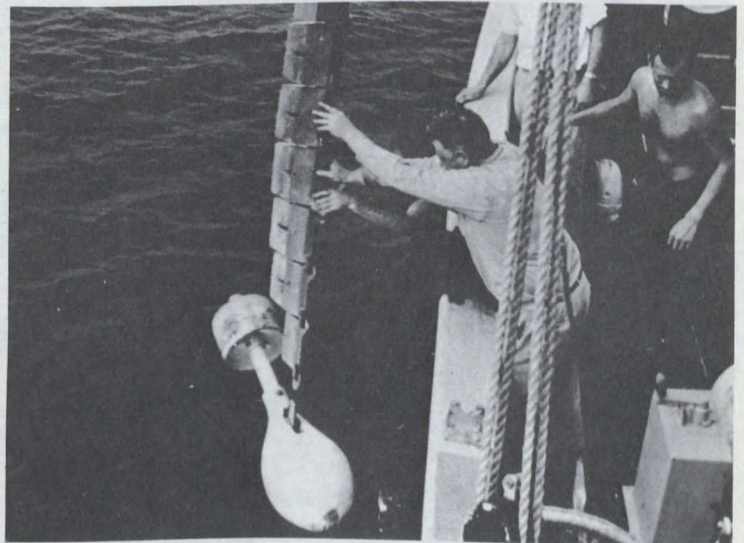
A shallow seismic profiler and underwater camera take the plunge.
