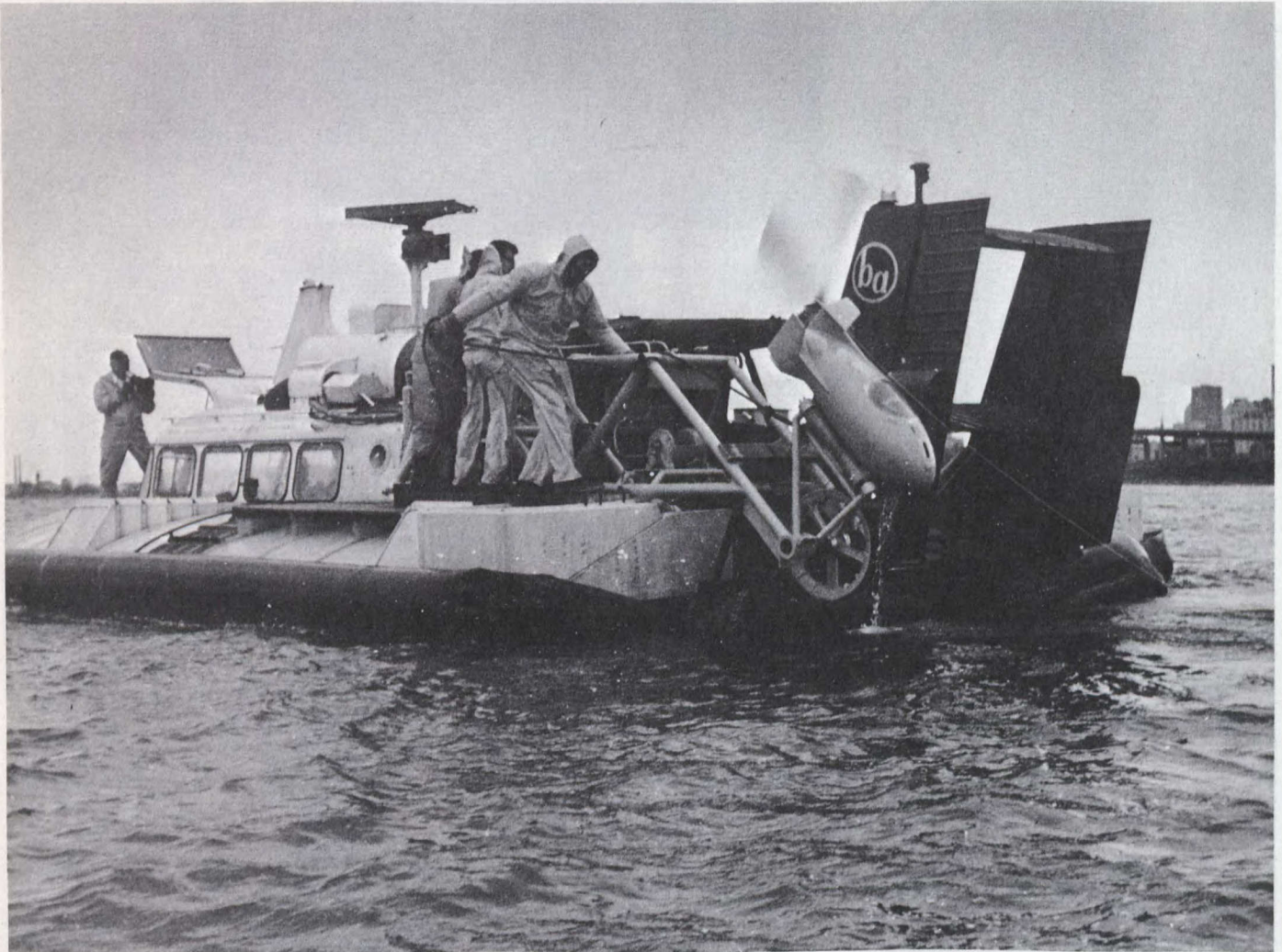
After completing a high-speed, deep underwater survey in the Great Lakes, a fully instrumented Fathom towed "fish" is brought aboard an SRN6 Hovercraft.
