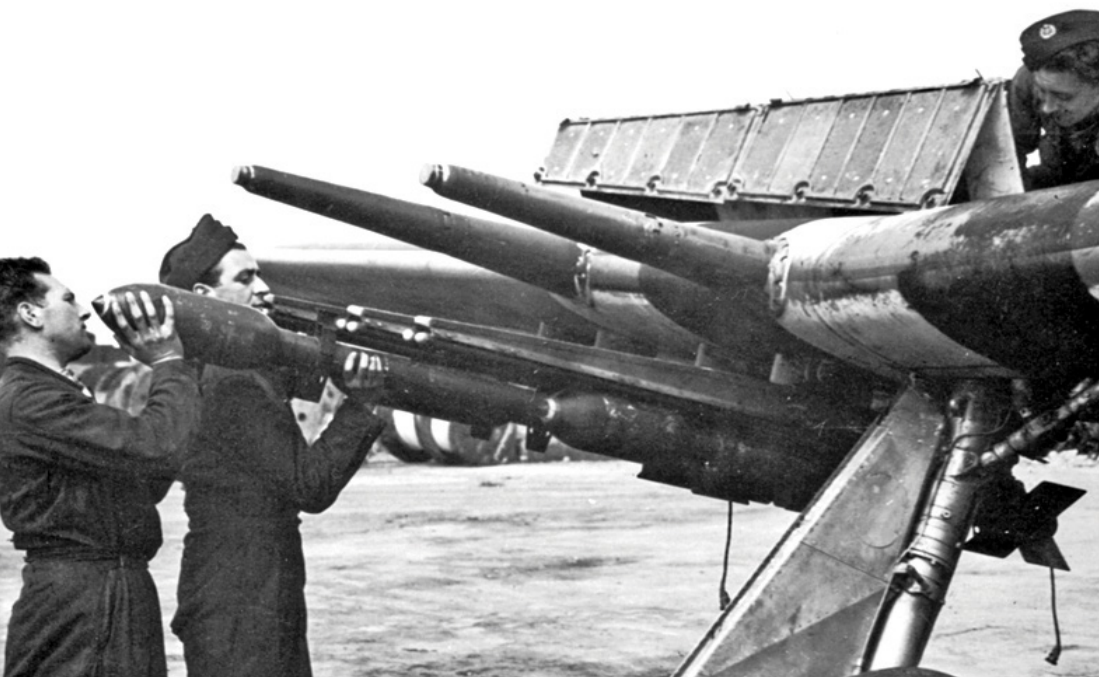
Armourers loading RP-3 rockets onto a Hawker Typhoon.
