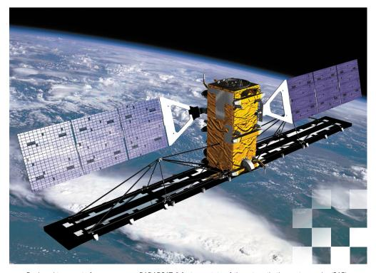
Designed to operate for seven years, RADARSAT-2 features state-of-the-art synthetic aperture radar (SAR) technology, and supports all the existing RADARSAT-1 beam modes while offering many powerful new capabilities.
