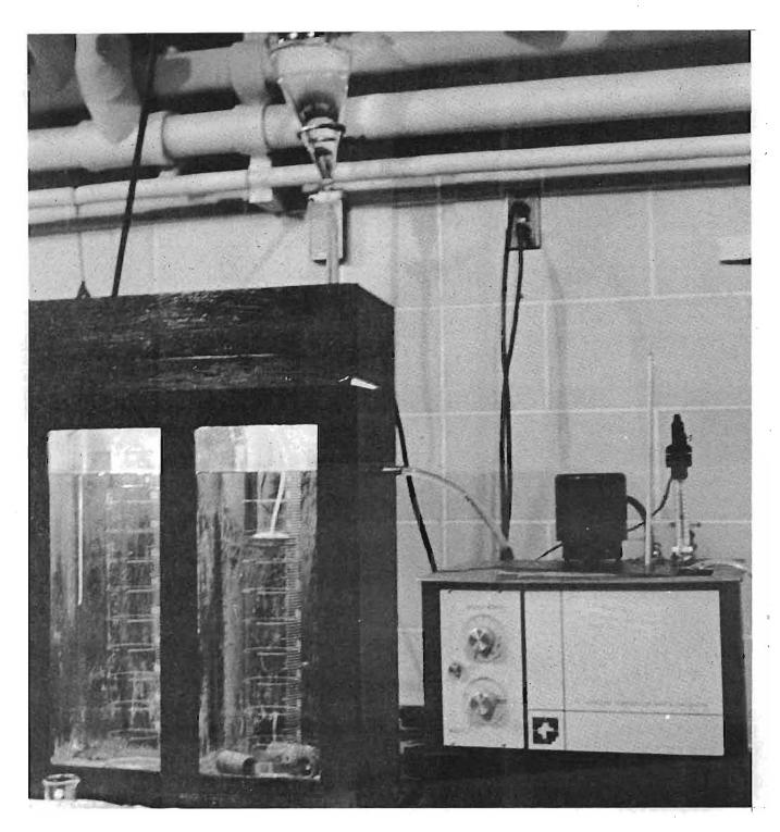
Fig. 1. General view of the Harder chamber and cooler. The right cylinder is being filled from the separatory funnel above but the top of the chamber is in its normal experimental position in order to illuminate the cylinders.
