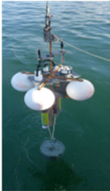
Figure 9. PAM mooring ready for deployment. The total height of the mooring is approximately 2 m.
