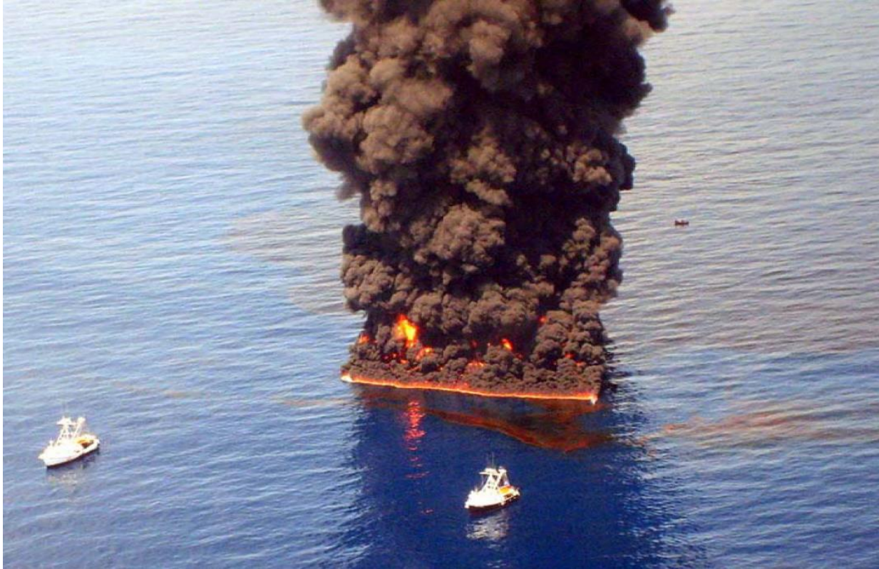
Figure 4. Ships towing booms feed oil into an in situ burn (Allen et al. 2011)
