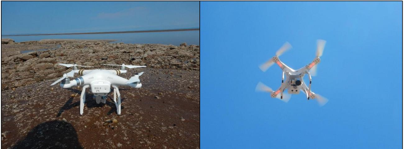
*Figure 1: Phantom 3 Professional from DJI, an off-the-shelf RPAS with a 12.4 megapixel camera.*
