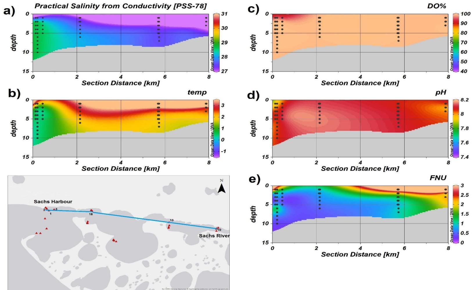
**Figure 5.** Cross section of water column properties between Sachs Harbour and mouth of Sachs River, NT, where section distance (km) starts at station 2. Profiles represent a) salinity (PSU), b) temperature ( $^{\circ}\text{C}$ ), c) dissolved oxygen (DO%), d) pH, and e) turbidity (FNU). Grey space represents the sea floor; specific values for each site can be found in Appendix B (stations 1, 2, 3, 18, 13 and 10).
