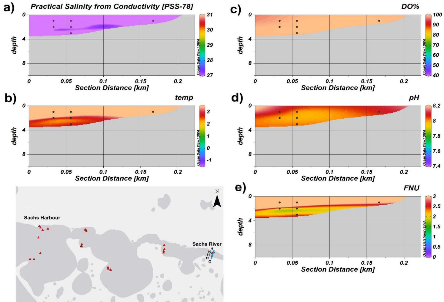
**Figure 11.** Transect G cross section of water column properties based on compiled YSI data. Profiles represent a) salinity (PSU), b) temperature ( $^{\circ}\text{C}$ ), c) dissolved oxygen (DO%), d) pH and e) turbidity (FNU). Grey space represents the sea floor; specific values for each site can be found in Appendix B (stations 9 to 11); section distance begins at station 9 on the northern shoreline.
