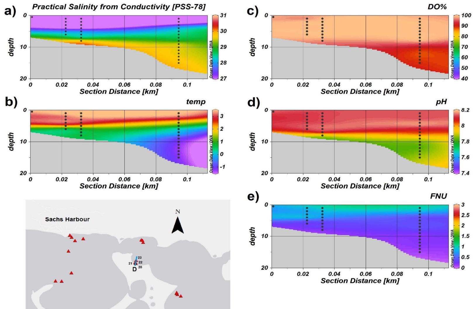
**Figure 8.** Transect D cross section of water column properties based on compiled YSI data. Profiles represent a) salinity (PSU), b) temperature ( $^{\circ}\text{C}$ ), c) dissolved oxygen (DO%), d) pH, and e) turbidity (FNU). Grey space represents the sea floor; specific values for each site can be found in Appendix B (stations 20 to 23); section distance begins at station 20, closest to the southern shore.
