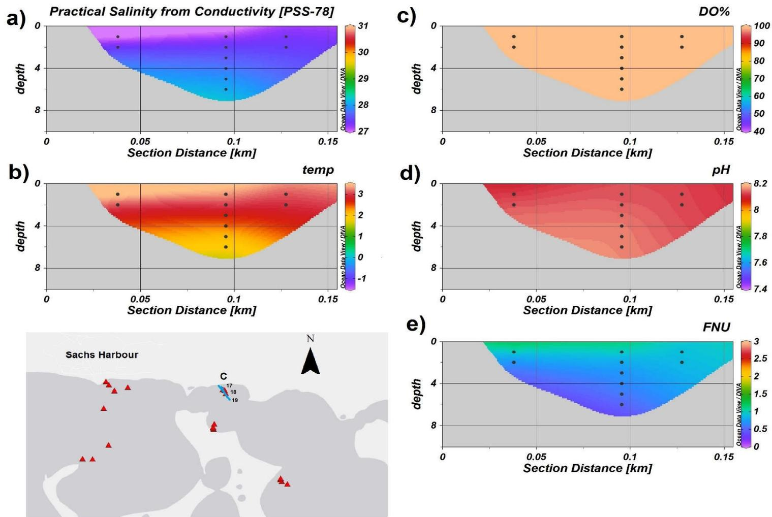
**Figure 7.** Transect C cross section of water column properties based on compiled YSI data. Profiles represent a) salinity (PSU), b) temperature (°C), c) dissolved oxygen (DO%), d) pH, and e) turbidity (FNU). Grey space represents the sea floor; specific values for each site can be found in Appendix B (stations 17–19); section distance begins at station 17 closest to the northern shoreline.
