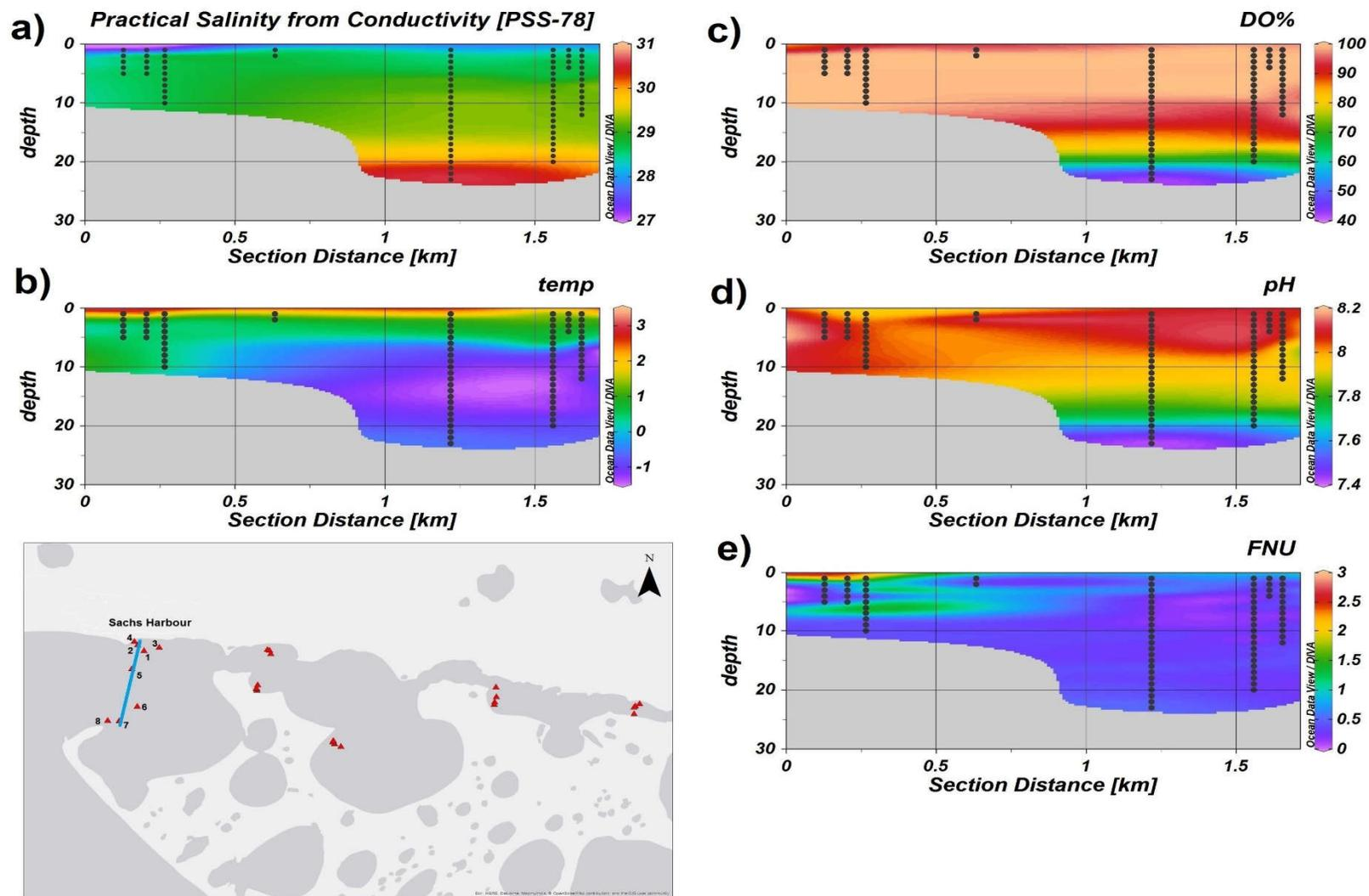
**Figure 6.** Transect B cross section of water column properties of a) salinity (PSU), b) temperature ( $^{\circ}\text{C}$ ), c) dissolved oxygen (DO%), d) pH, and e) turbidity (FNU); specific values for each site can be found in Appendix B (stations 1–8). Section distance starts at station 4, closest to the hamlet of Sachs Harbour.
