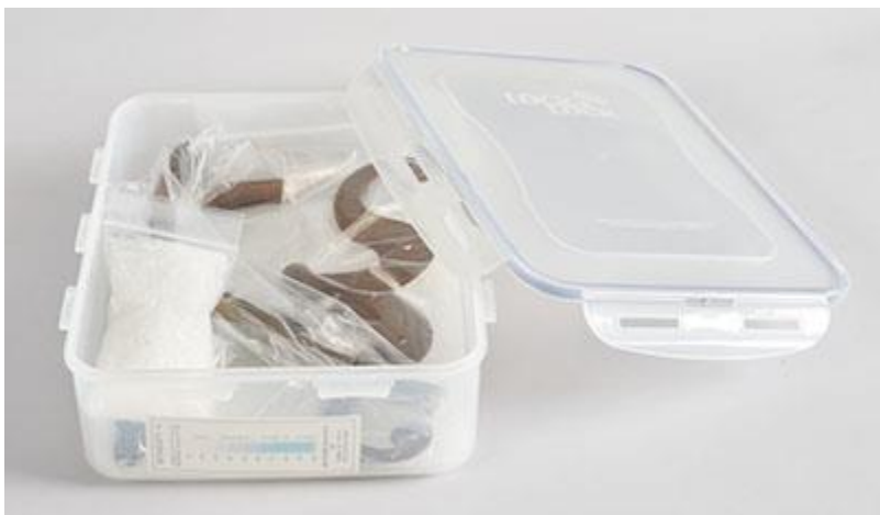
Figure 13. These iron objects are packed for dry storage in a food container with silica gel and an RH indicator card.
