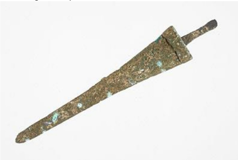
Figure 11. Corroded iron. Archaeological iron that is contaminated with salt is particularly vulnerable to elevated or fluctuating humidity levels.
