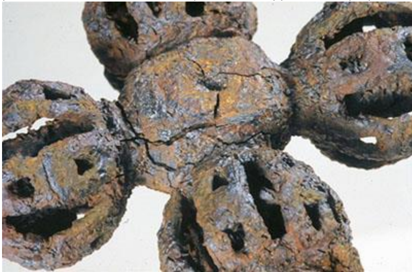
Figure 18. Detail of cracking caused by active corrosion after excavation.
