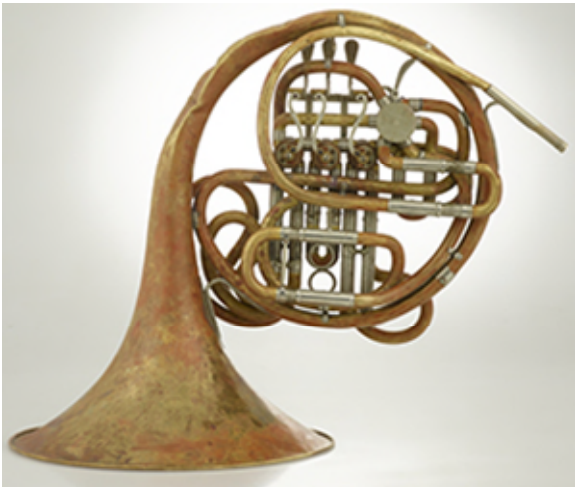
© Government of Canada, Canadian Conservation Institute. CCI 129915-0003 Figure 2. French horn (made circa 1966), showing pink areas typical of dezincification.
