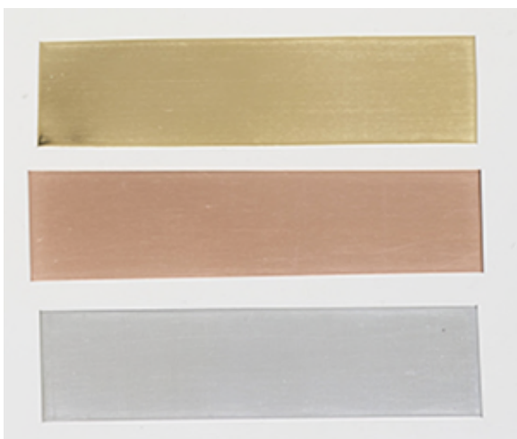
© Government of Canada, Canadian Conservation Institute. CCI 129915-0014 Figure 1. From top to bottom: cartridge brass, pure copper and pure zinc.
