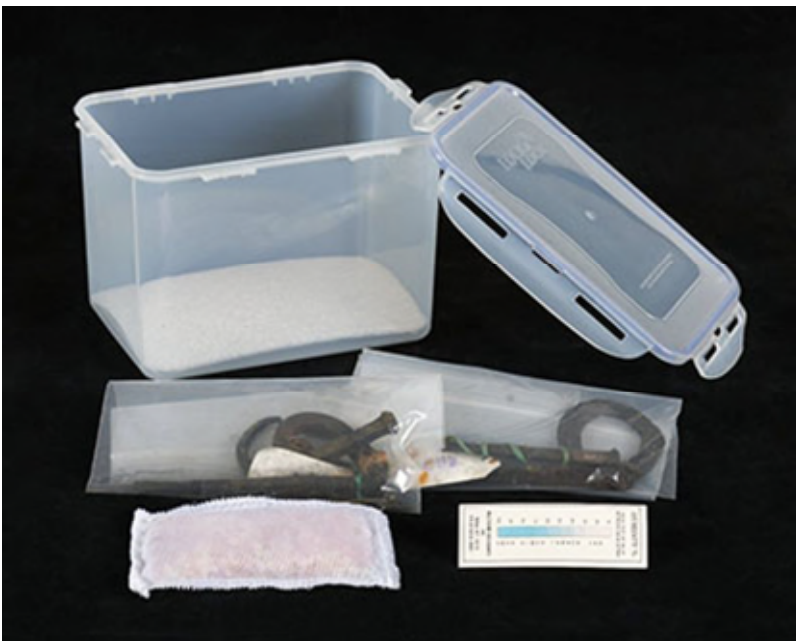
© Government of Canada, Canadian Conservation Institute. CCI 126258-0001 Figure 2. Lock & Lock box with iron objects, silica gel and humidity indicator card.
