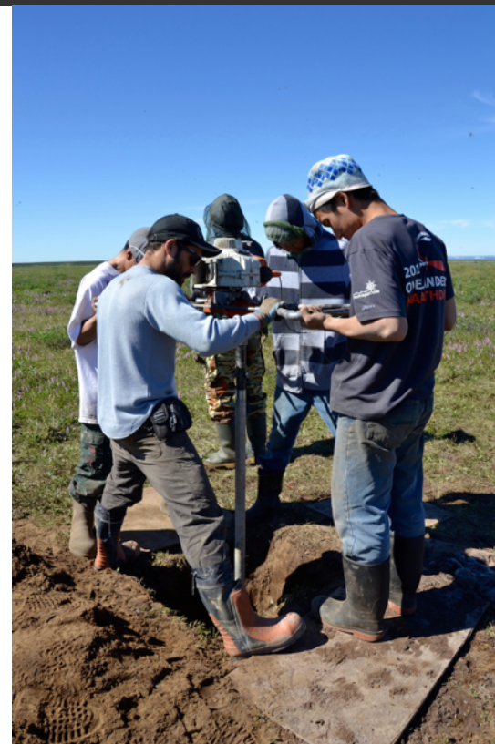
Permafrost coring in Kugluk Territorial Park, Nunavut
