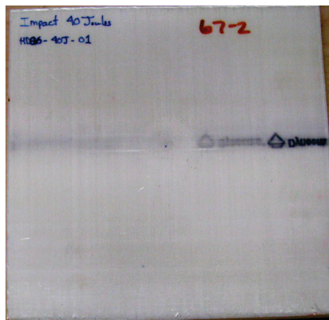
Figure 2: Photograph of a 40J impacted UHMWPE panel.
