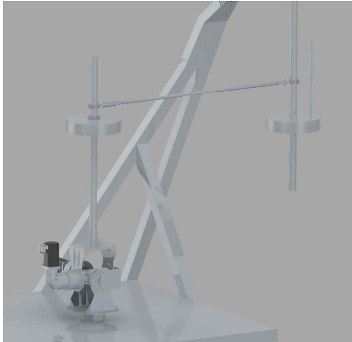
Figure 51: Implementation of the tension/compression link with the pendulating load model.
