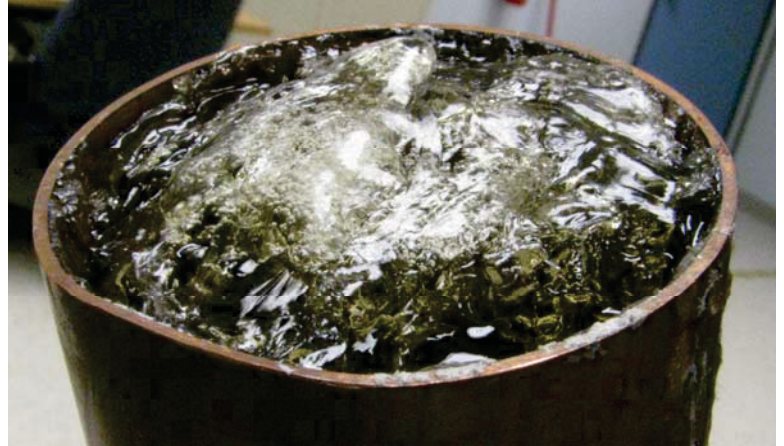
Figure 89. Copper pipe filled with solethane compound - view 2.
