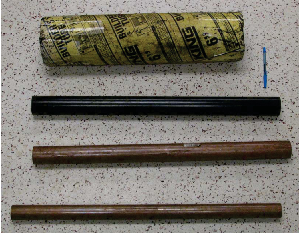
Figure 33. Cylinders used as tunnel surrogates.
