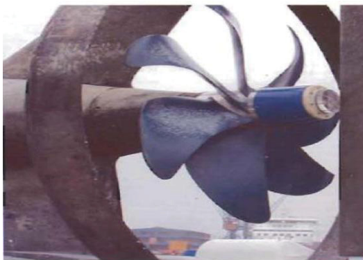
(a) Composite propeller installed on 206A Class submarines
