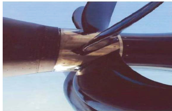
(b) Composite propeller installed on 212A Class submarines
