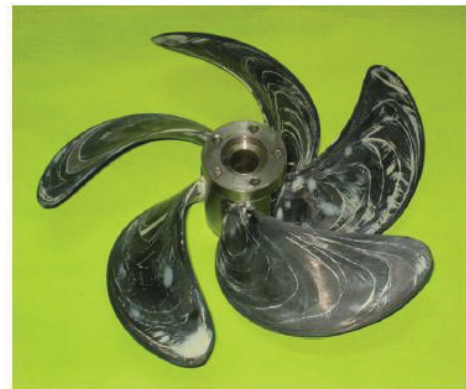
(b) Mould, Composite Blade, and Assembled Composite Propeller
