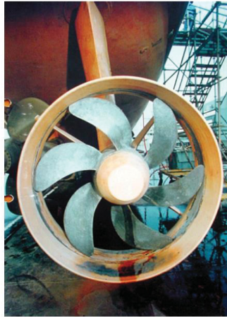
Figure 11: Contur Carbon Fibre Propellers Fitted on a Mine Hunter of Netherlands Navy.
