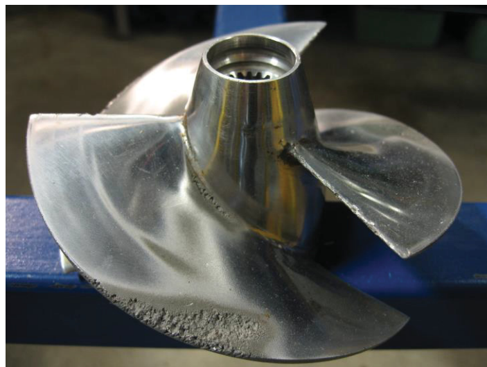
Figure 2: Illustration of Cavitation Damage in Metallic Propeller.
