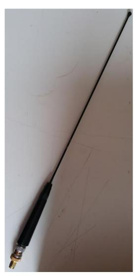
Figure 2. Monopole antenna.
