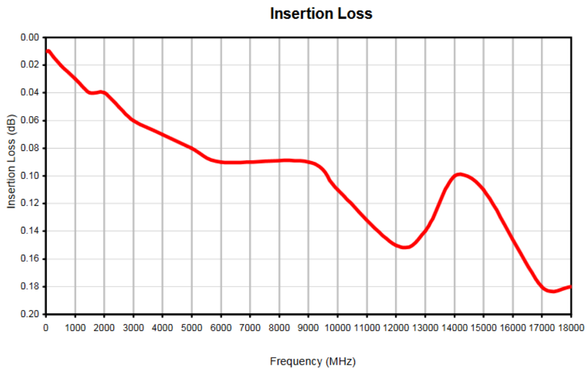
Figure 1. NF-SF50+ Adapter Insertion Loss (Mini-Circuits 2014).
