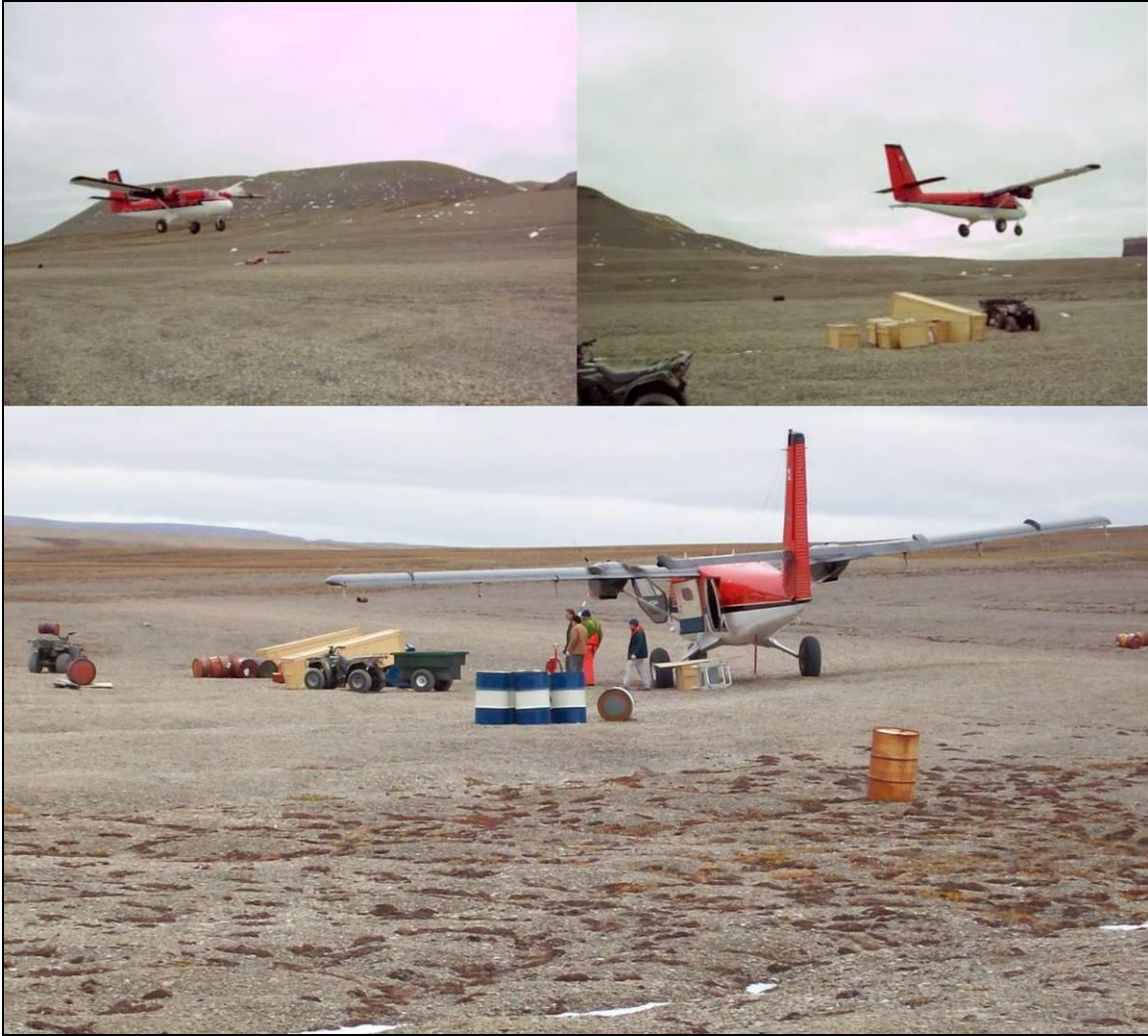
Figure 19: Short gravel runway at Gascoyne Inlet used by DRDC to access a small camp there. The special tires of the Twin Otter allow it to easily land and take off from such a rough strip consisting of sharp broken shale, with numerous depressions like the one in the foreground [photos by D. Brookes, 2008]
