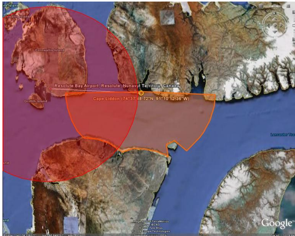
Figure 22: The estimated coverage zone (shaded orange) for a 25 kW marine navigation radar situated on top of Cape Liddon at 320m above sea level compared to the nominal communications range (shaded red) for a ScanEagle or Integrator UAV with a base station at Resolute. The radar coverage is based on a marine target with a Radar Cross Section (RCS) of about 75 dBsm 16 .
