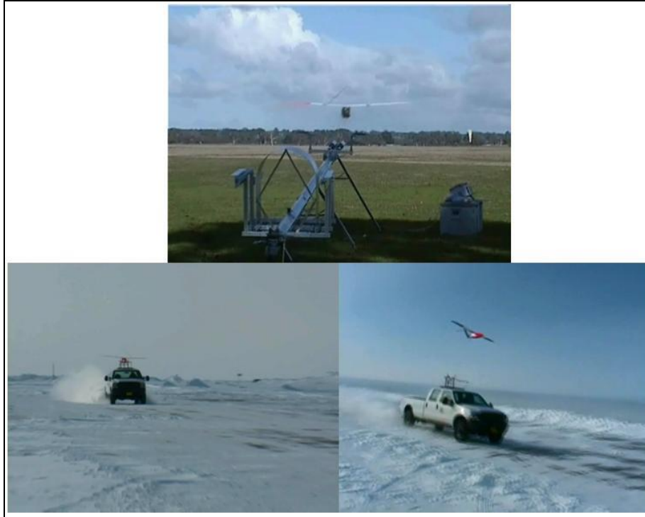
Figure 54: Aerosonde launch options: via a launch catapult (upper) or ground vehicle; recovery is by belly landing. [Photos are screen captures from an Aerosonde promotional video [44]]
