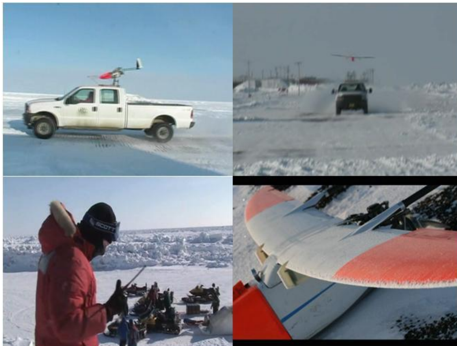
Figure 55: Cold weather operation testing in Barrow, Alaska: over 1000 h of successful operation [Screen captures from an Aerosonde promotional video [44]].
