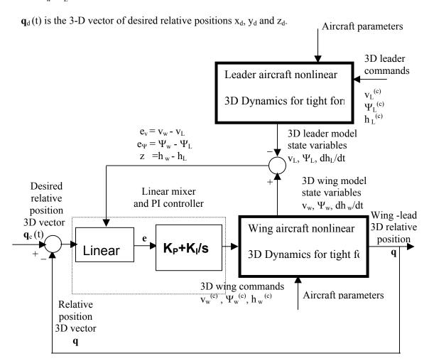
Fig. 3.19 Block diagram for the PI control of the relative distance between two aircrafts in tight formation flight
