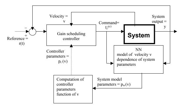
Fig. 3.8 Heading controller using gain scheduling based on a Neural Networks model
