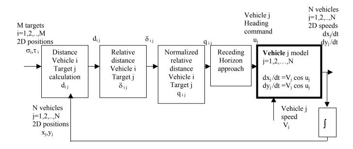
Fig. 4.6 Generic diagram for MPC for heading control of multi-vehicles and multitargets
