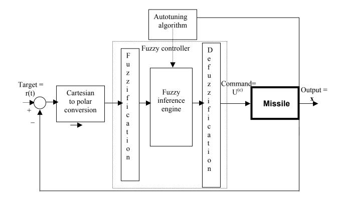
Fig. 3.12 Autotuned fuzzy controller for guidance
