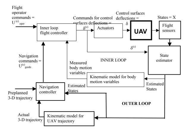
Fig. 3.1 UAV advanced flight controller structure
