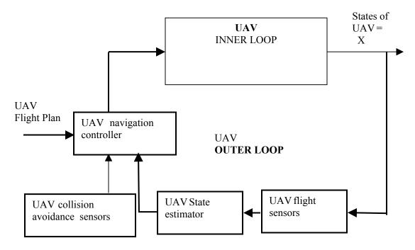
Fig. 2.5 Outer loop controller system
