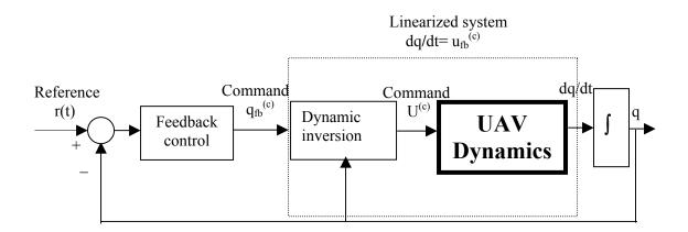
Fig. 4.4 1D dynamic inversion of UAV flight dynamics
