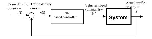
Fig. 3.5 Traffic flow controller using Neural Networks
