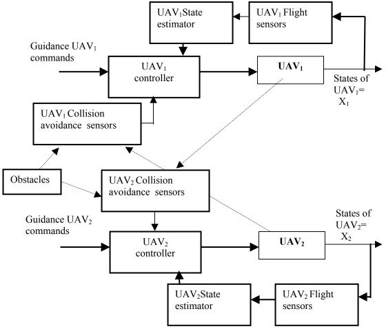
Fig. 3.20 Sensing-communication requirements for control of multi UAVs
