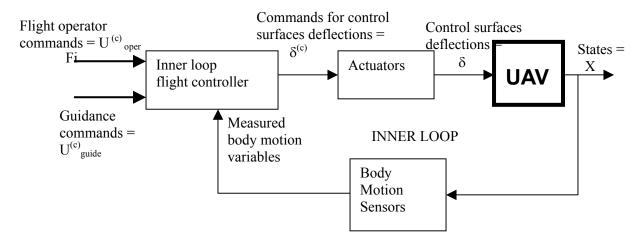
Fig. 2.1 Inner loop control system
