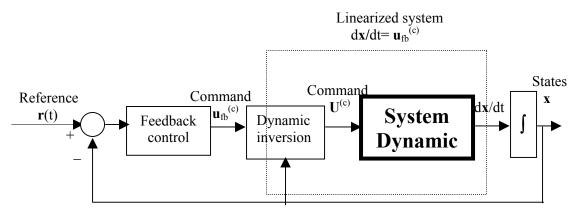
Fig. 4.3 Generic diagram for dynamic inversion
