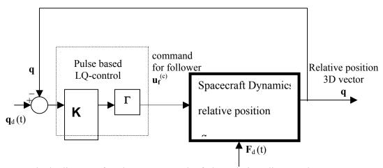
Fig. 3.18 Block diagram for the LQ control of the relative distance between two spacecrafts
