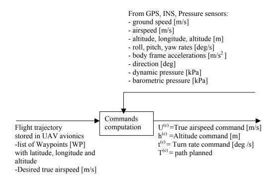
Fig. 2.7 UAV commands computation
