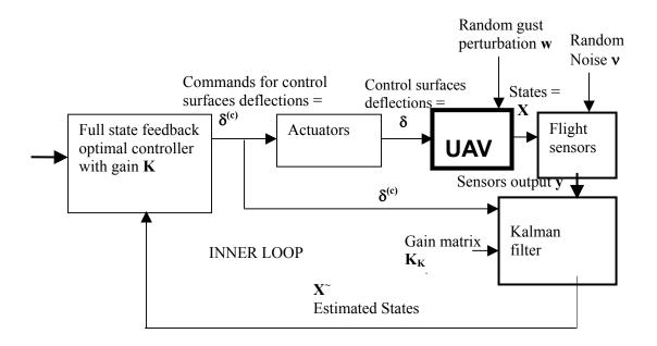
Fig. 3.3 LQG optimal controller for the inner loop
