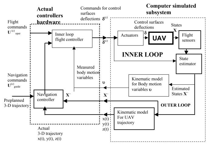
Fig. 4.7 Generic block diagram of a conventional HIL simulation setup
