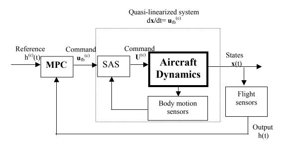
Fig. 4.5 Generic diagram for MPC for path-flight control
