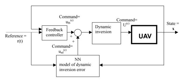
Fig. 3.9 UAV flight control using a Neural Network
