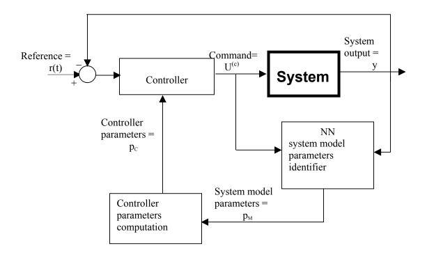
Fig. 3.7 Self-tuning regulator using a Neural Networks model
