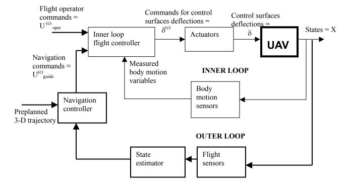
Fig. 1.1 UAV conventional flight control system
