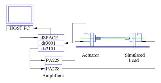
Figure 4.9 HIL setup with simulated load
