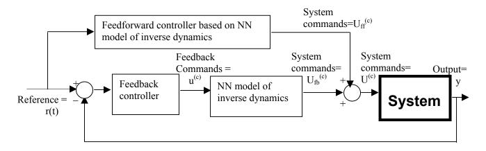
Fig. 3.4 Generic block diagram of a controller using Neural Networks (NN)
