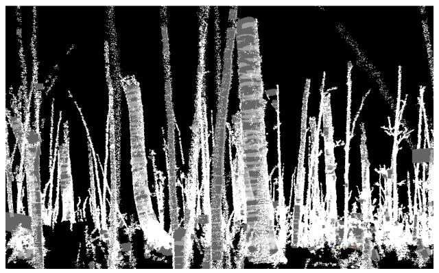
A ground-based image captured by LiDAR (Light detection and ranging), used for precise estimates of forest parameters such as volume, stem form, and stand density.
