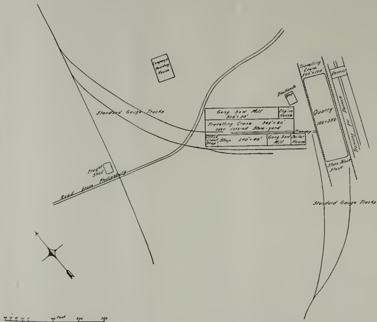
FIG. 8. Plan of the quarry, mills, and yards of the Missisquoi Marble Co., Phillipsburg, Que.
