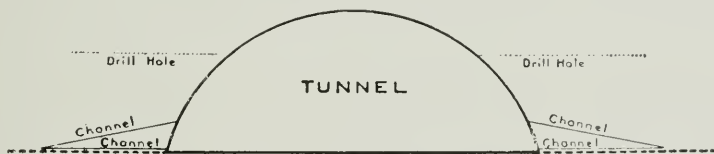
FIG. 7. Method of extending a tunnel laterally.
