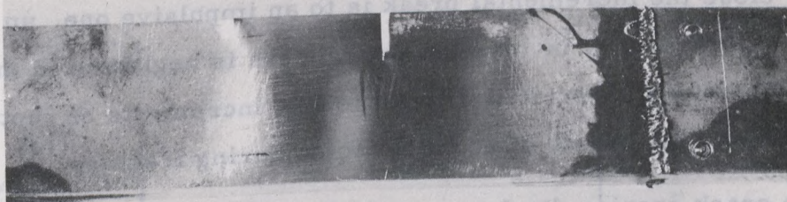
Figure 7. Irregular yield zone at root of notch of 1/4 in. thick specimen tested at -75^{\circ}\text{C} .
