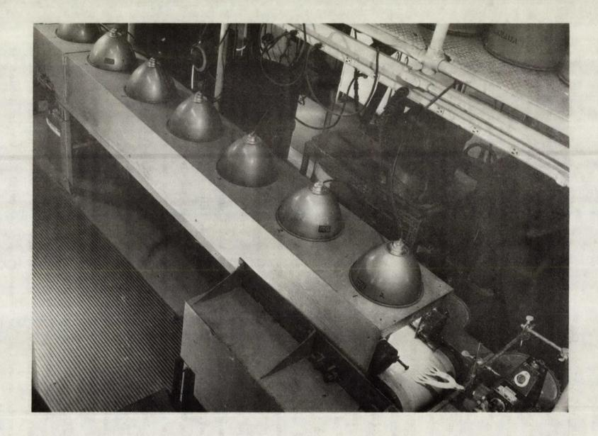
Figure 1 - A photograph of the conveyor belt and tunnel used for continuous drying on a pilot-plant scale.
