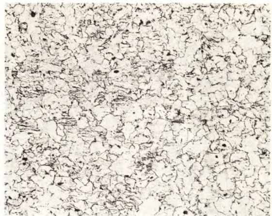
(b) Seamless Tubing DT (rimmed steel)
