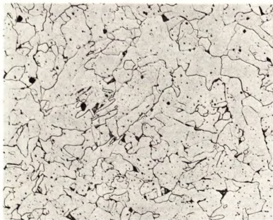
(c) Welded Tubing ET (rimmed steel)
