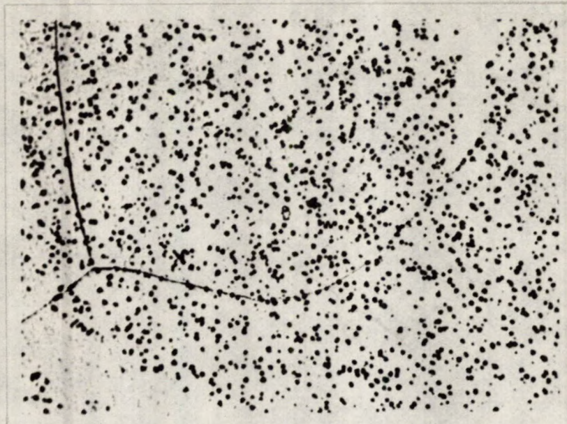
Figure 7: Zr-1.0%Cu-1.5%Mo. Quenched from 1000°C (1830°F), aged 500°C (930°F) for 48 hr. As polished.
