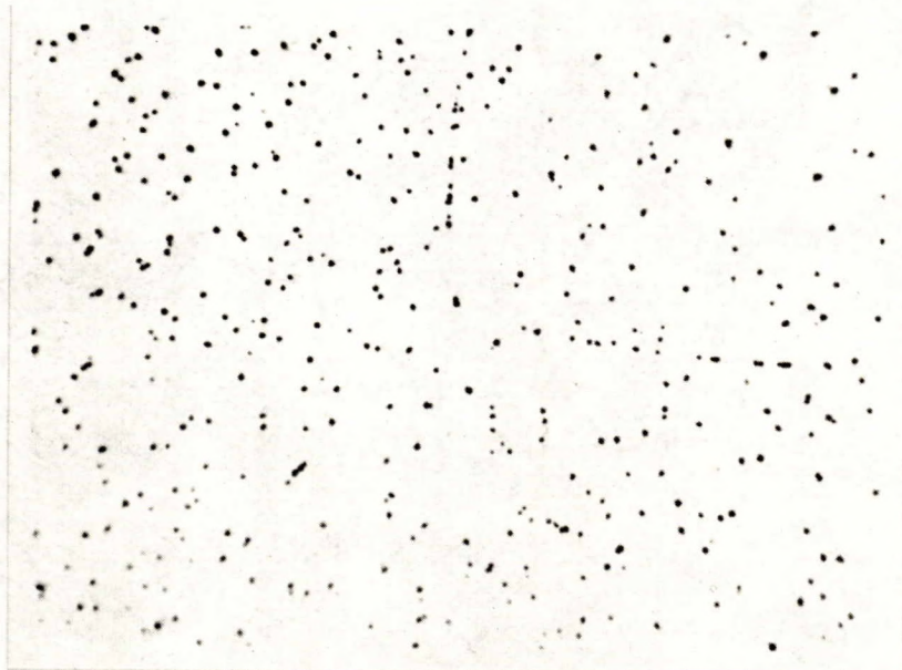
Figure 5: Zr-1.0%Cu-1.5%Mo. Quenched from 1000°C (1830°F), aged 500°C (930°F) for 30 min. As polished. Oblique illumination.
