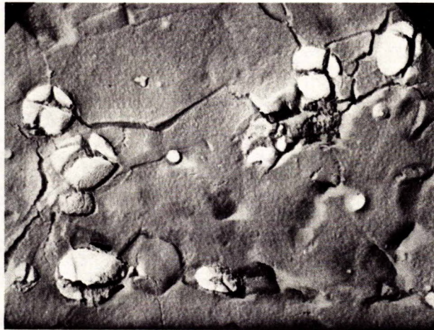
Figure 32: Zr-0.5%Cu-0.5%Mo. Annealed 700°C (1290°F) 1 hr; corrosion-tested 24 hr.
