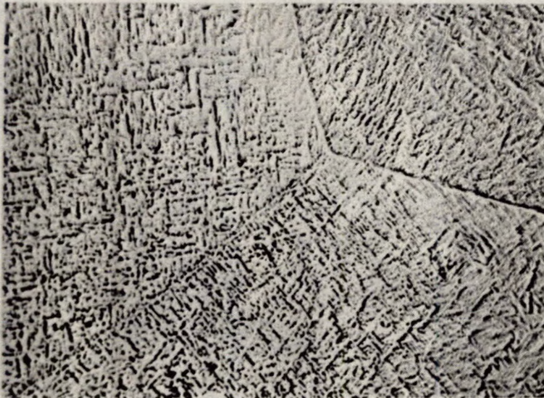
Figure 3: Zr-1.0%Cu-1.5%Mo. Heat-treated 900°C (1650°F), WQ. As polished.
