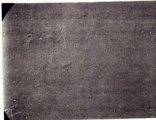
Figure 25: Zr-0.5%Cu-0.5%Mo. Quenched from 1000°C (1830°F), aged 500°C 8 hr. As polished.
