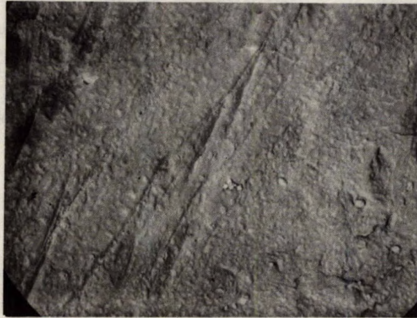
Figure 30: Zr-0.5%Cu-0.5%Mo. Quenched from 1000°C (1830°F), aged at 500°C for 24 hr; corrosion-tested 24 hr.
