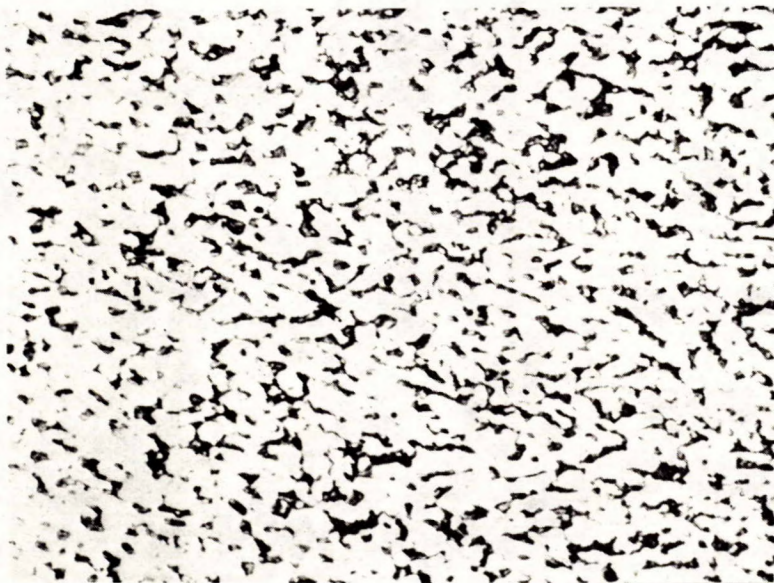
Figure 10: Zr-1.0%Cu-1.5%Mo alloy (ICI). Heat-treated 1000°C (1830°F) 1 hr, WQ, aged 500°C (930°F) 100 hr. Etched for Zr-Cu phase.
