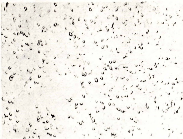
Figure 9: Zr-1.0%Cu-1.5%Mo alloy (ICI). Heat-treated 1000°C (1830°F) 1 hr, WQ, aged 500°C (930°F) 100 hr. Etched for Zr-Mo phase.
