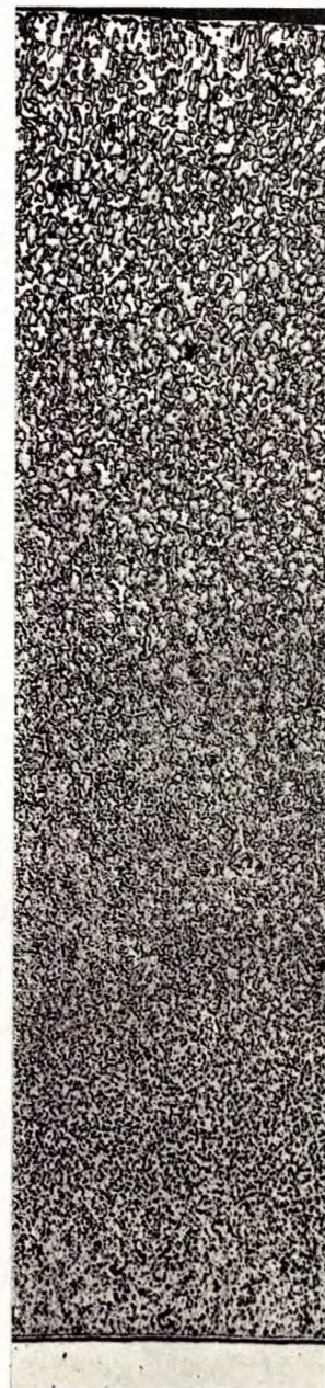
Figure 15. Coatings on electropolished faces of Cambridge (110) iron crystal as indicated: 2.5-min immersion at 450°C (840°F). X200.
