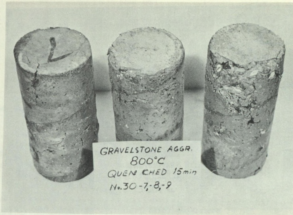
A. Cracked and disintegrated cylinders, retaining only 15% of original strength.
