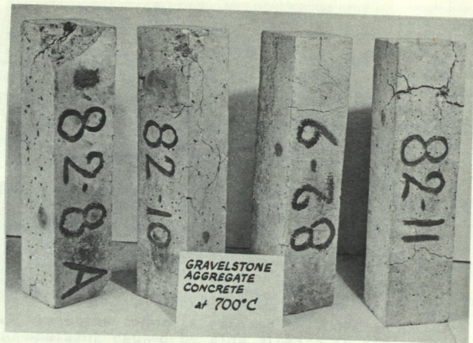
A. Extensive cracking of concrete beams caused by expanding aggregate particles.
